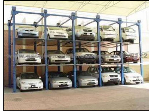
Gambar 15. Contoh puzzle parking system Sumber: Indiamart, 2011
