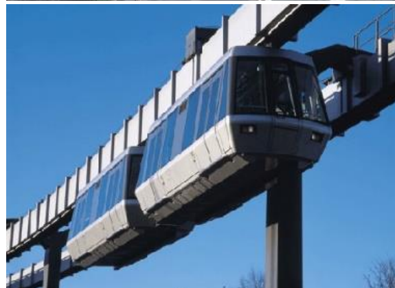
Gambar 2. Straddle beam dan suspended monorel Sumber: The Monorail Society
