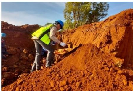
Gambar 1. *Sampling test pit*
