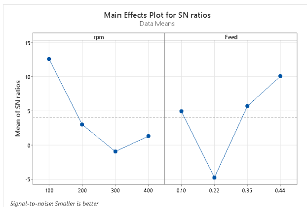
Gambar 5 . Main effects plot for SN ratios (vibration amplitude)
