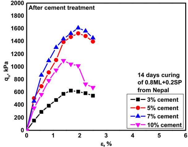
Fig. 15. Undrained strength of cement treated red soil mixed with poorly graded gravelly sand, 14 days curing.
