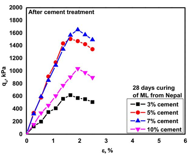
Fig. 13. Undrained strength of cement treated red soil, 28 days curing.
