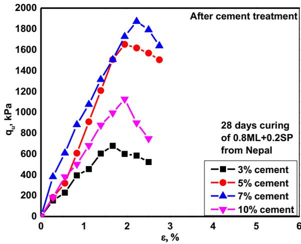
Fig. 16. Undrained strength of cement treated red soil mixed with poorly graded gravelly sand, 28 days curing.
