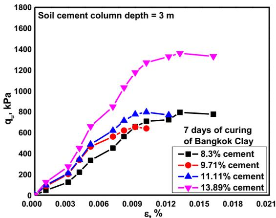
Fig. 4. Undrained strength of treated Bangkok Clay (7 days curing).
