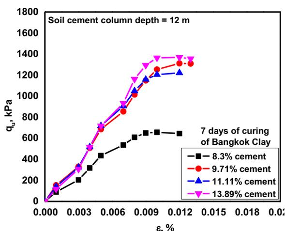
Fig. 7. Results of undrained strength of cement treated Bangkok Clay of 7 days curing at 12.0 m depth.
