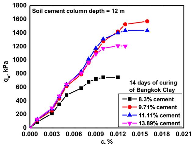
Fig. 8. Undrained strength of cement treated Bangkok Clay, 14 days curing at 12.0 m depth.
