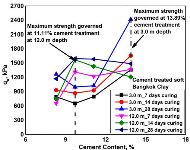
Fig. 19. Representation of maximum strengths received after curing soft Bangkok Clay of Thailand.
