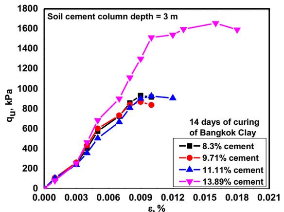
Fig. 5. Undrained strength of treated Bangkok Clay (14 days curing).
