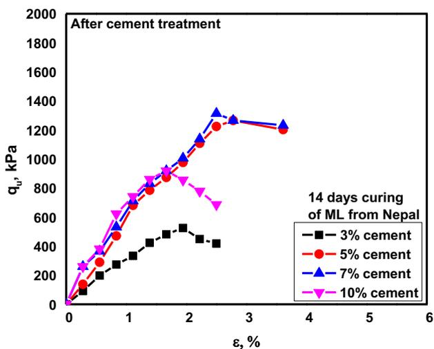
Fig. 12. Undrained strength of cement treated red soil, 14 days curing.
