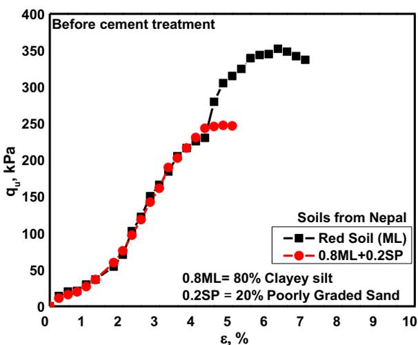
Fig. 10. Undrained strength of red soil and mixed with poorly graded soil.
