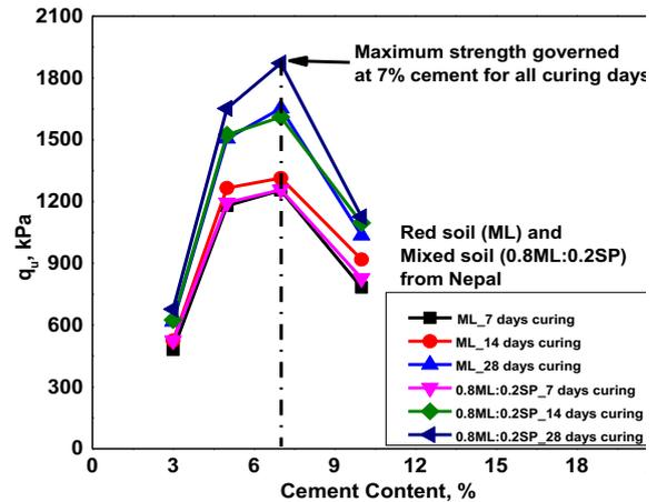
Fig. 20. Representation of maximum strengths received after curing red soil of Nepal.
