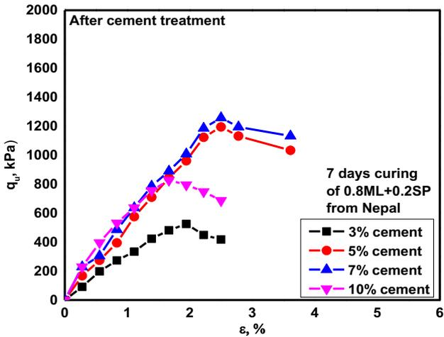
Fig. 14. Undrained strength of cement treated red soil mixed with poorly graded gravelly sand, 7 days curing.
