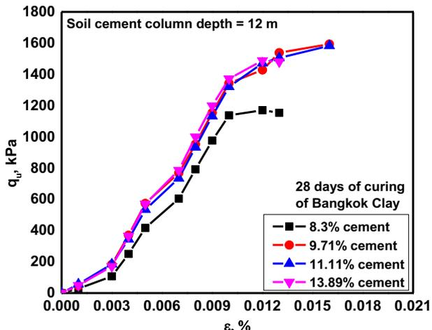
Fig. 9. Undrained strength of cement treated Bangkok Clay, 28 14 days curing at 12.0 m depth.
