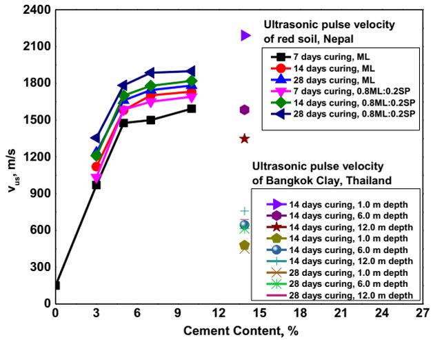
Fig. 17. ultrasonic pulse velocity versus cement content of Bangkok Clay and mixed soil from Nepal.
