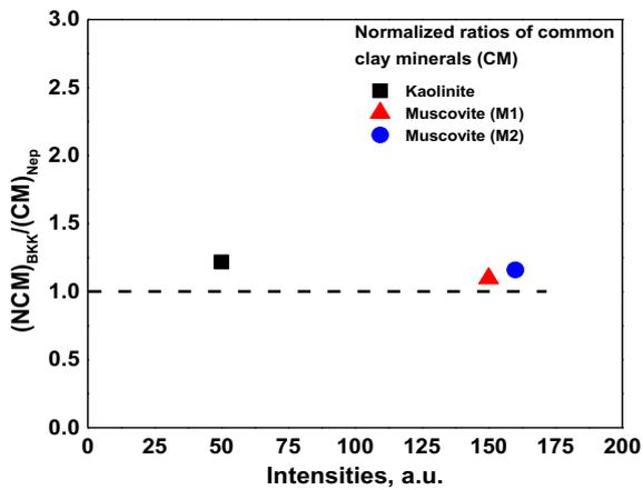
Fig. 18. Normalized clay minerals of soft Bangkok Clay with reference to clay mineral from red soil of Nepal.
