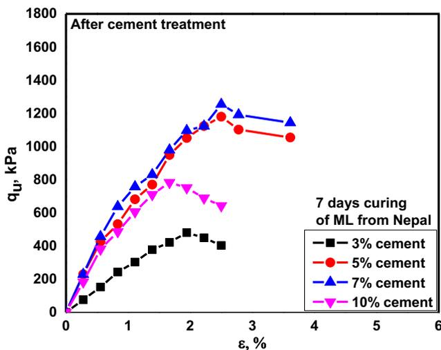
Fig. 11. Undrained strength of cement treated red soil, 7 days curing.
