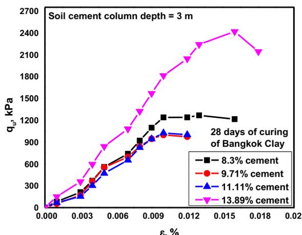
Fig. 6. Results of undrained strength of cement treated Bangkok Clay of 28 days curing.
