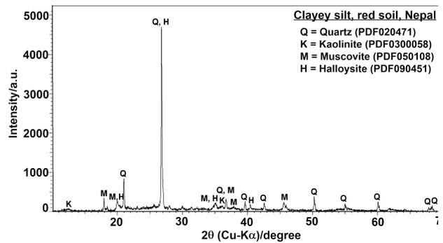
Fig. 3. Representation of XRD results of red soil (ML), Nepal
