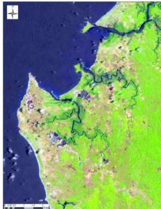
Fig. 6. True colour composite image of a Coastal Zone in Myanmar, produced by combining Sentinel-2 multispectral bands Red, Green and Blue within ArcGIS.
