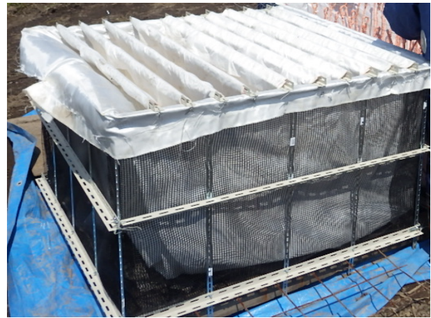
Fig. 9. Field setup with non-woven geotextile (cloth)
