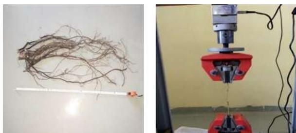
**Fig.1** Tensile strength testing machine and sample prepared for testing.
