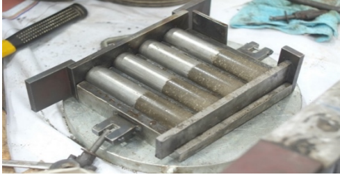
Fig. 5. Samples preparation of 3.5 cm diameter and 7.0 cm height
