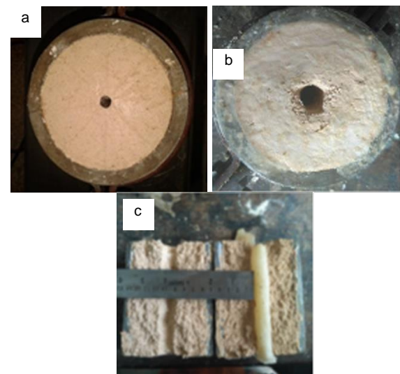
Fig.2 (a) Sample before test with 6mm hole (b) Sample(C10) which showed very less surface erosion after HET when coated with wax on its surface (c) Cross section of a sample after HET
