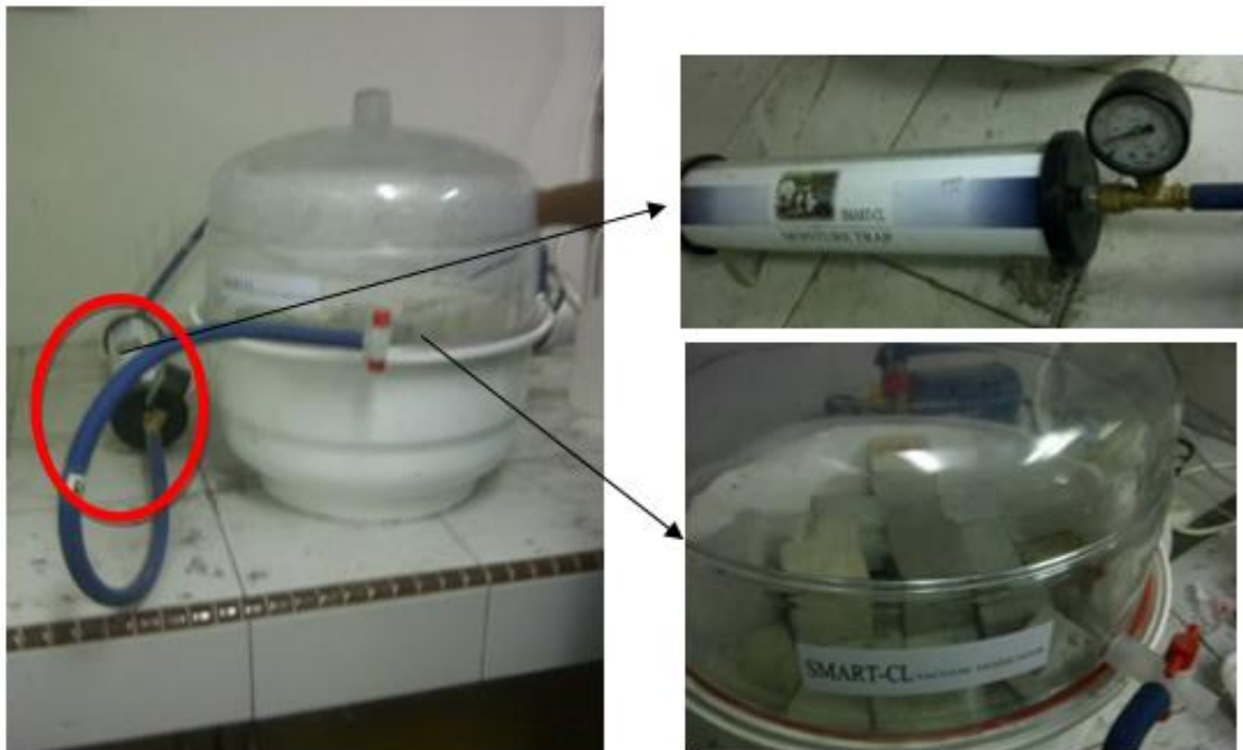
Fig. 7. Porosity test using SMART-CL vacuum dessicator with moisture trap
