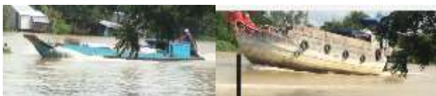
Pointed bow ship Blunt bow ship Fig 4. Pointed bow and blunt bow ship
