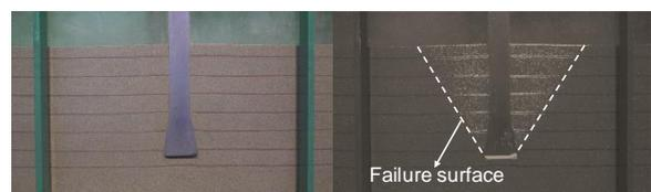
**Fig.2.** A Study on the Failure Surface of Bell Type Pile Model Test Using Image Analysis.
