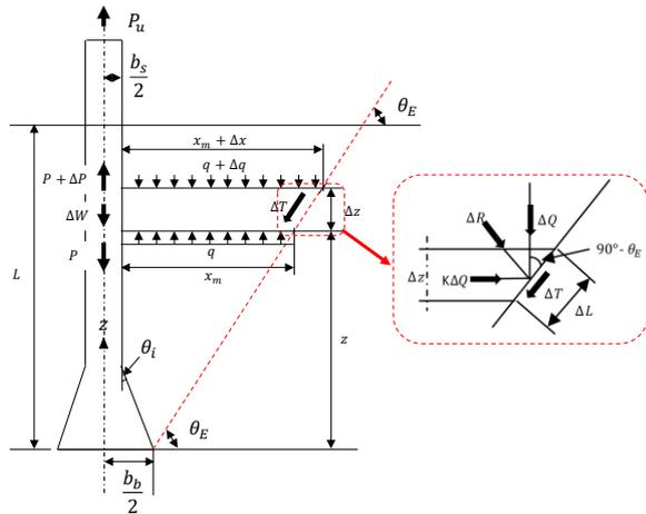
**Fig. 3.** A Study on the failure surface of belled-type pile model experiment using image analysis
