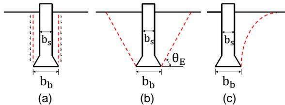
**Fig. 1.** Assumed failure mechanisms for belled piles subject to uplift loads.
