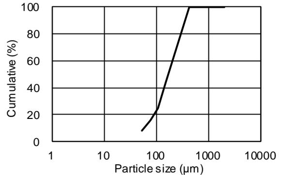
Fig. 6. Particle size distribution curve (USCS)
