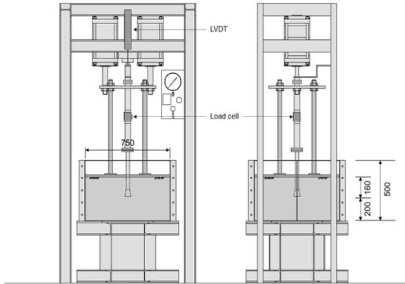
Fig. 4. Model experiment apparatus
