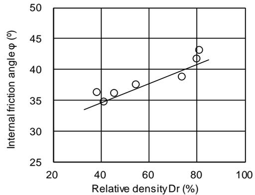
**Fig. 10.** Direct shear test on relative density
