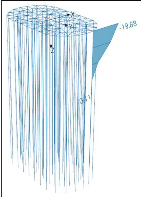
Fig 14. Pile cap horizontal displacement (stage 2)
