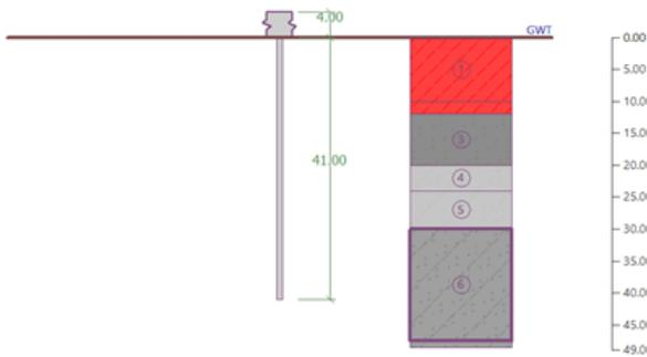
**Fig 9.** Stage 3 Soil Profiles
