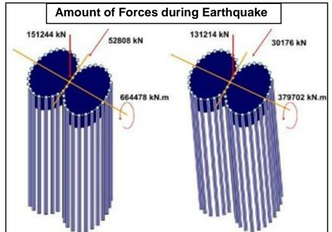
**Fig 12.** Pile group loads (without pile cap weight)
