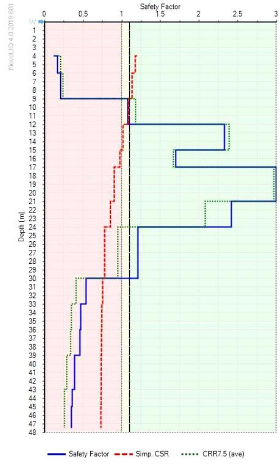
**Fig. 4.** Safety Factor (Mw = 7.7)
