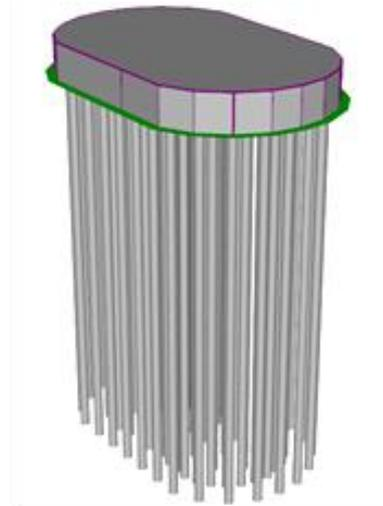
**Fig 11.** Pile cap of phylon Ir. Soekarno cable-stayed bridge
