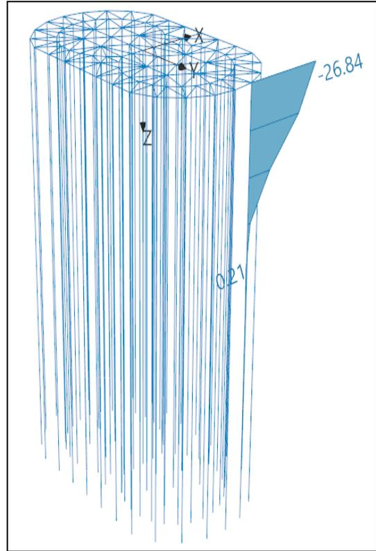
Fig 15. Pile cap horizontal displacement (stage3)
