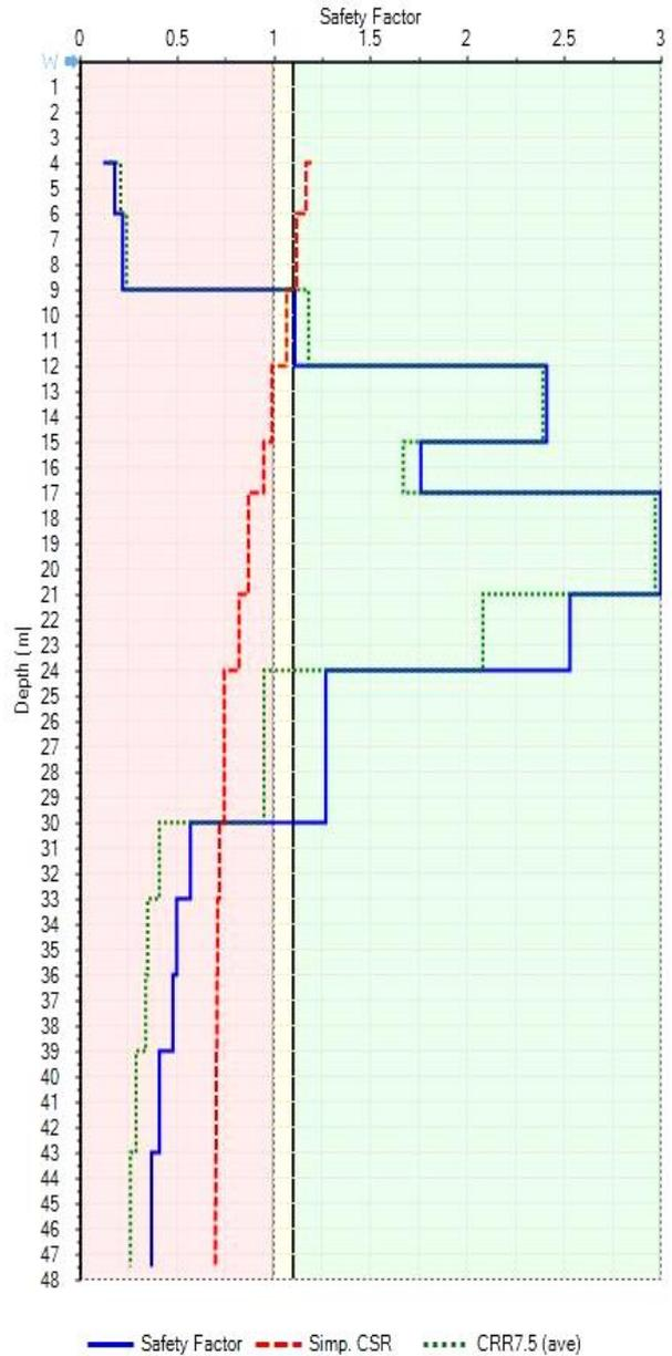
Fig. 2. Safety Factor (Mw = 7.5)
