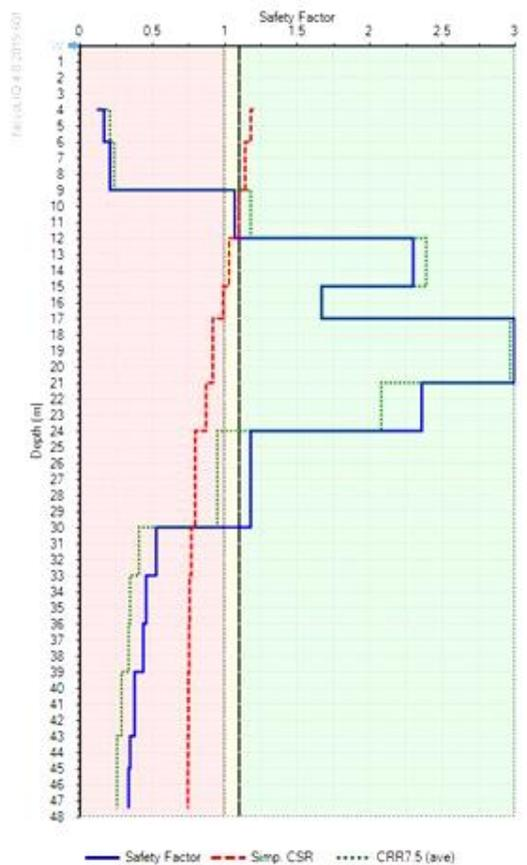
**Fig. 5.** Safety Factor (Mw = 7.8)
