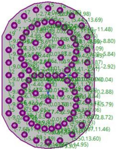
**Fig 10.** Pile group alignment
