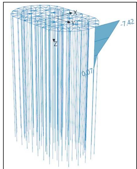
**Fig 13.** Pile cap horizontal displacement (stage 1)
