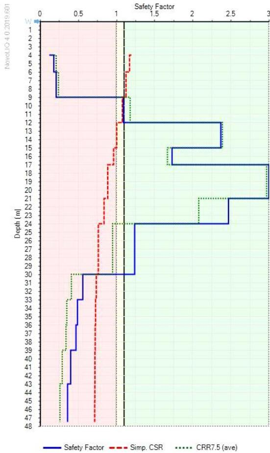
**Fig. 3.** Safety Factor (Mw = 7.6)
