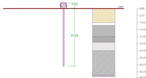
**Fig 7. Stage 1 Soil Profiles**
