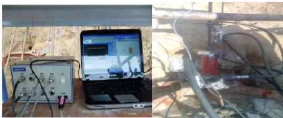
Fig.14d. Pullout test soil nail
