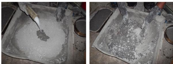
Fig. 3. Sample preparation for unconfined compressive strength (UCS) experiment
