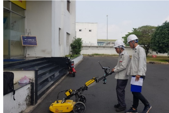
Fig. 1. A GPR machine survey, IDS Detect Duo, Italy
