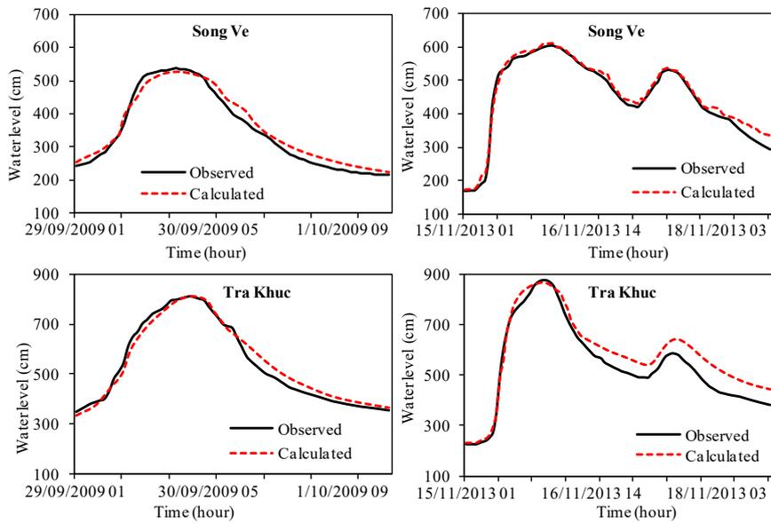
Fig. 7. Validation of water level at Song Ve and Tra Khuc station in 2009 and 2013.
