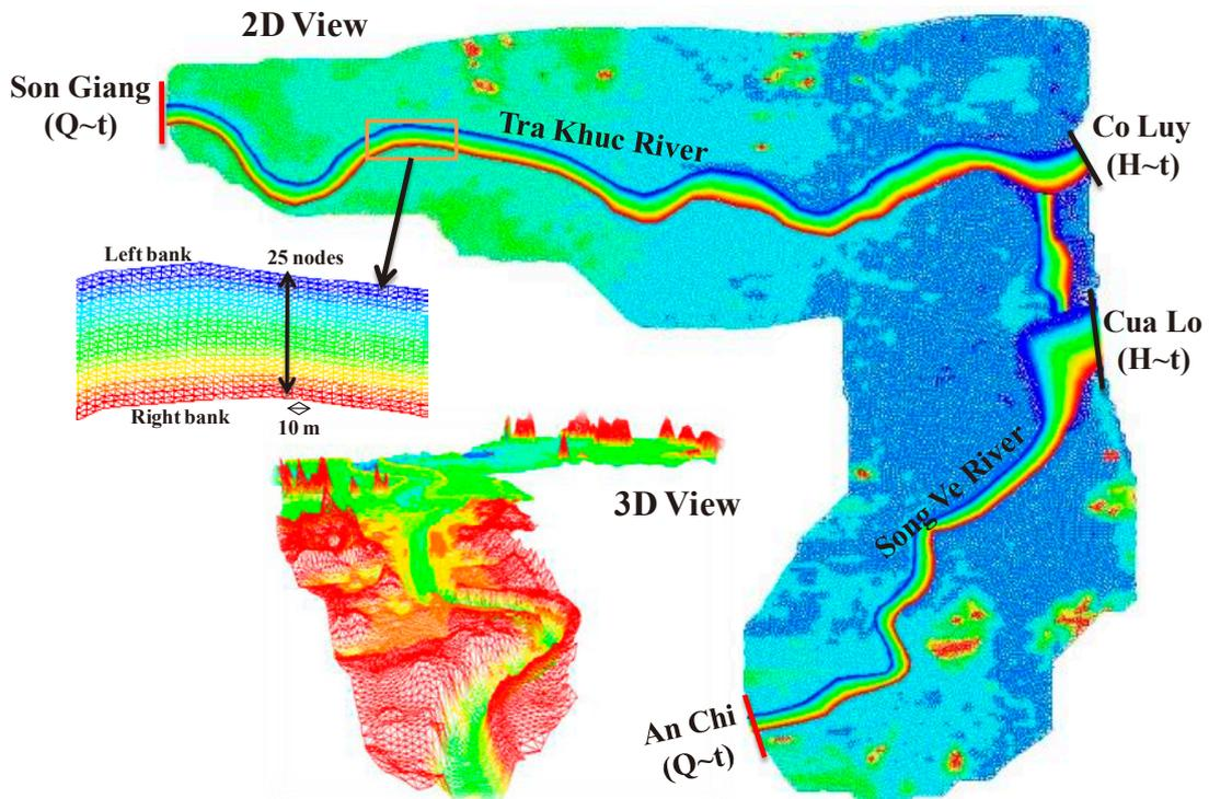
Fig. 5. Bathymetry mesh 2D, 3D in BlueKenue.
