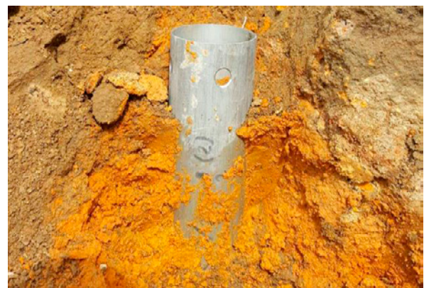
Fig. 7. Collecting volcanic soil using steel tube sampler.
