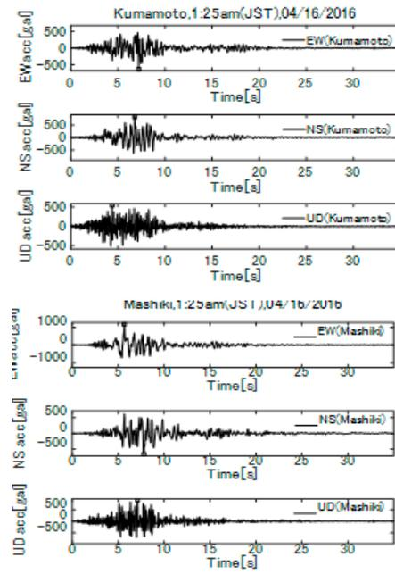
**Fig. 6.** Ground motion during the main shock (Source: KikNet and JMA).
