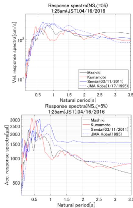
**Fig. 8.** Acceleration and velocity spectra of the main shock (Source: KikNet and JMA).
