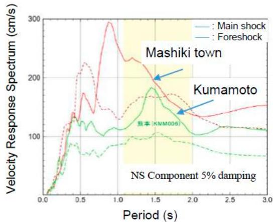
**Fig. 9.** Comparison of the velocity spectra of the two events (Source: ERI, University of Tokyo).
