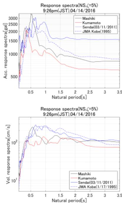
**Fig. 7.** Acceleration and velocity spectra of the foreshock (Source: KikNet and JMA).
