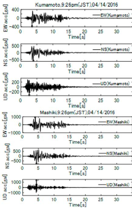
**Fig. 5.** Ground motion due to foreshock of April 14 (Source: Kik-net and JMA).
