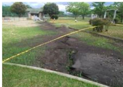
**Fig. 5.** Fissure ejecting black sand along former river (Kojima Park, Nishi-ku, Kumamoto City, 32.776476N, 130.635140E)
