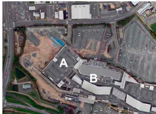
(b) After the main shock of April 16 (Geospatial Information Authority of Japan, 2016). Building A and B with spread foundation were settled due to liquefaction.
