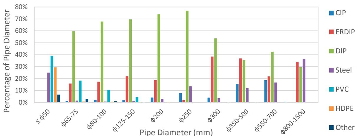
**Fig. 6.** Percentage of pipe by diameter used in Kumamoto City.
