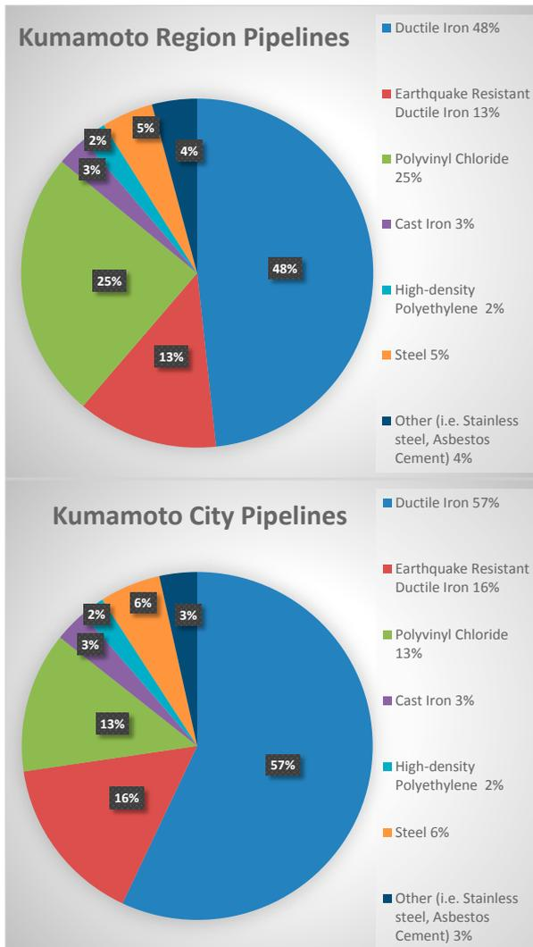
**Fig. 4.** Distribution of water supply pipelines (untreated, transmission, and distribution mains) in Kumamoto Region and Kumamoto City (data from JWVA, 2014).
