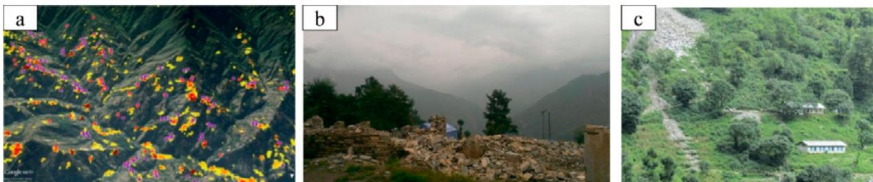
**Fig. 17.** (a) Ridge-top damage interpreted from satellite image decorrelation before and after the main shock (ARIA/JPL-Caltech), (b) a completely destroyed school on the hill top (N:27.837392°, E:85.854154°), and (c) an intact school at the hill valley near the school on the hill top (N:27.804319°, E: 85.913725°) (Sharma and Deng, 2017).
