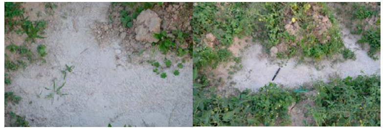
Fig. 33. Observed local scale liquefied white colored fine silty sand at the agricultural field in Imadol area.
