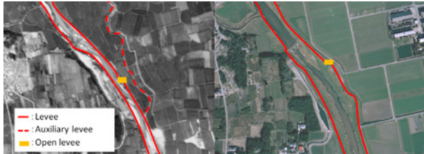
Fig.3 Plan views of Jobaru River before (left) and after (right) the disaster subsidy project
