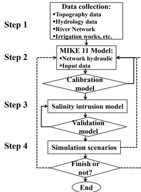
Fig. 4. Calculation procedures of the simulation.
