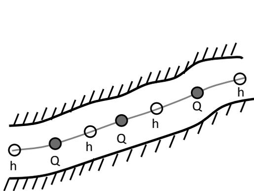
Fig. 2. Schematic nodding of h-points and Q-points for a river section MIKE 11 mode (Eaton and Franson, 2005).
