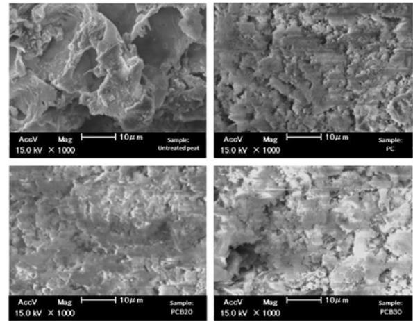
Fig. 3. Scanning Electron Microscope (SEM) on untreated (above left) and stabilized peat (PC: above right, PCB20: below left, PCB30: below right).
