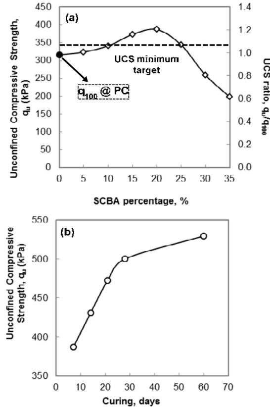
Fig. 2. (a) Effect of SCBA percentage replacement on the UCS of the stabilized peat; (b) Effect of optimum PCB mixture on the UCS at various curing durations.
