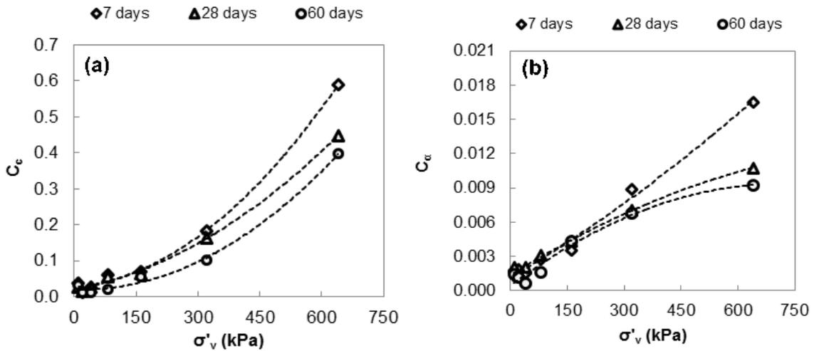
Fig. 6. The variation of compression index,  $C_c$  and coefficient of secondary compression,  $C_\alpha$  with applied effective stress at different curing times on PCB20 mixture.
