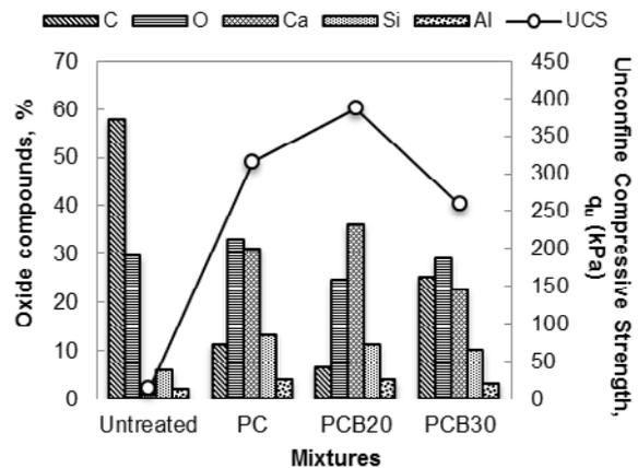
Fig. 4. Summary of crucial oxide compound percentages of untreated and stabilized peat from EDX test.
