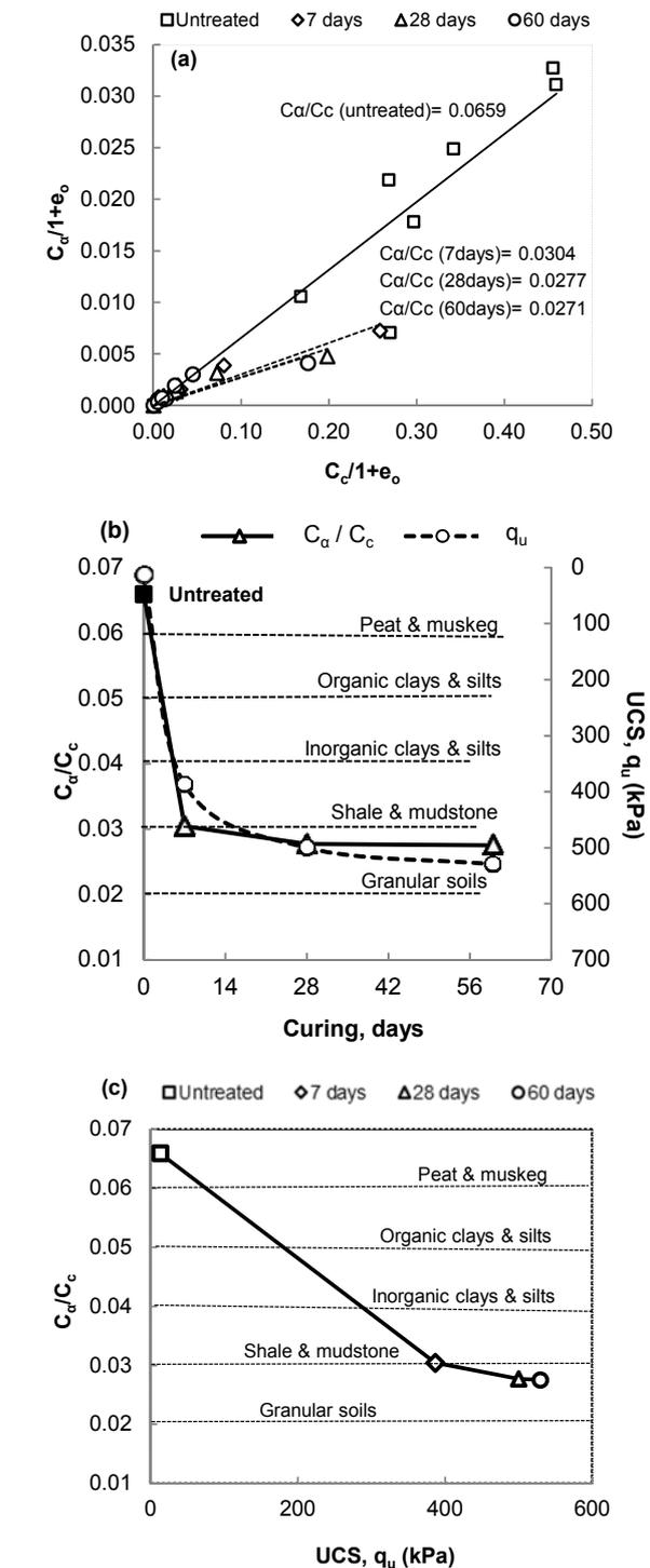
**Fig. 7.** The variation of compression index ratio,  $C_{\alpha}/C_c$  untreated and PCB20 mixture at different curing times.
