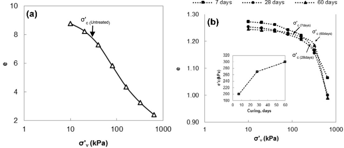
Fig. 5. Void ratio ( $e$ ) versus effective vertical stress ( $\sigma'_v$ ) for; (a) untreated peat; (b) PCB20 mixture at 7, 28 and 60 days of curing.
