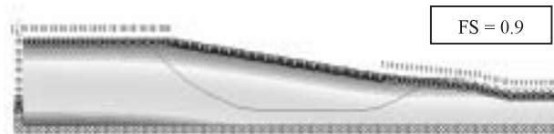
Fig. 7 Stability analysis for natural riverbank using LEM - Slide 5
