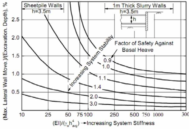
Fig. 1 Design chart for estimating maximum lateral wall movement in soft to medium clays (Clough and O'Rourke 1990)
