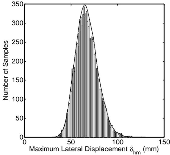
Fig. 3 Histogram of estimated maximum wall deflection using KJHH model (Case No. 5)
