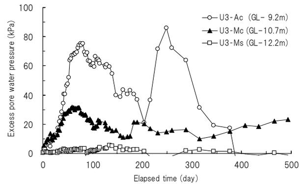
Fig. 8 Measured excess pore water pressure
