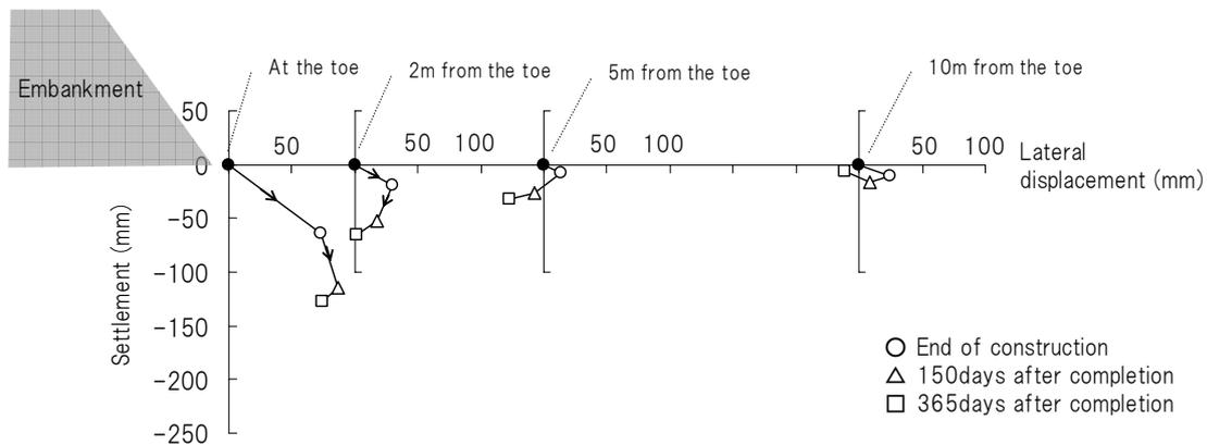
Fig. 10 Measured surface deformation in surrounding area
