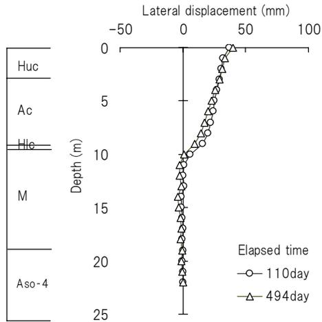
Fig. 9 Measured lateral displacement profiles
