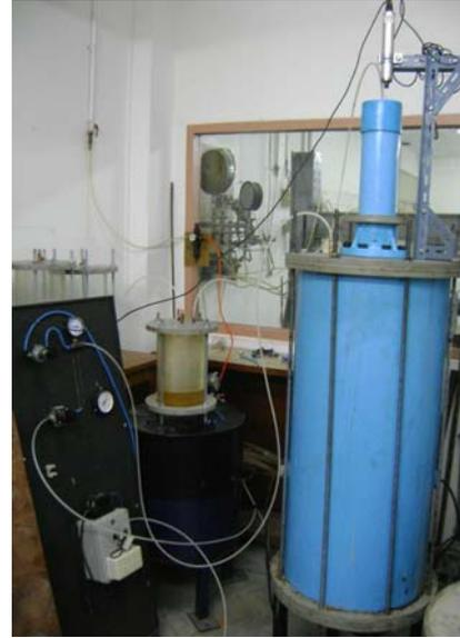
Fig. 1 Large scale consolidometer
