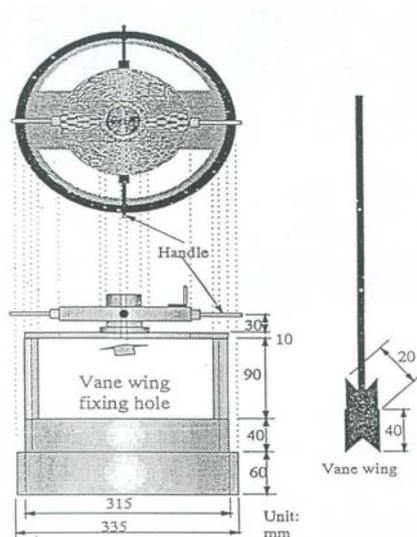
Fig. 3 Schematic of laboratory vane shear apparatus
