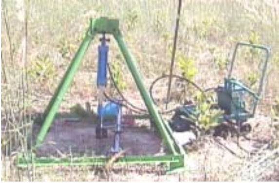
Fig. 9 Large scale field pullout test
