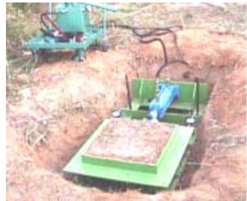
Fig. 18 Large scale direct field shear test
