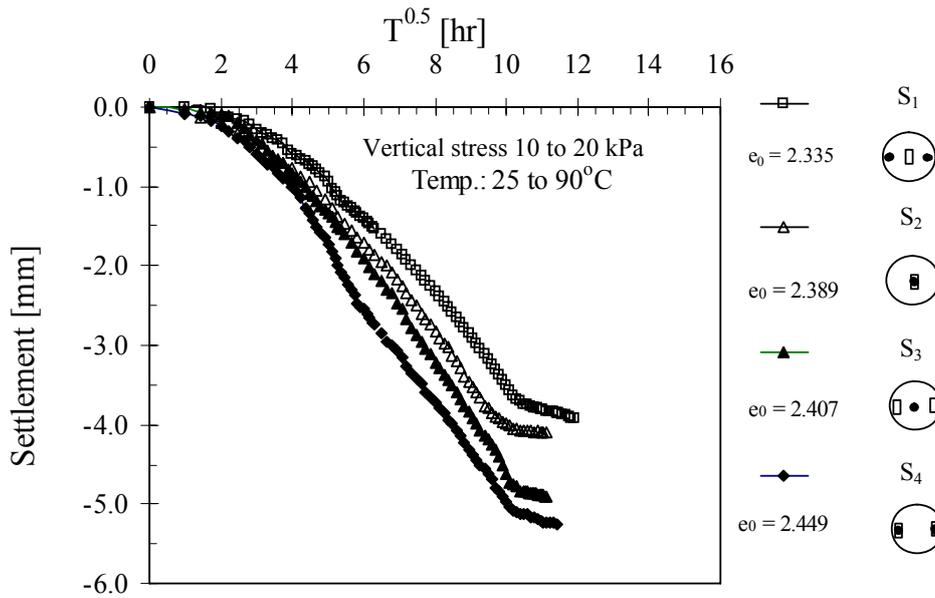
Fig. 11 Thermal consolidation test results
