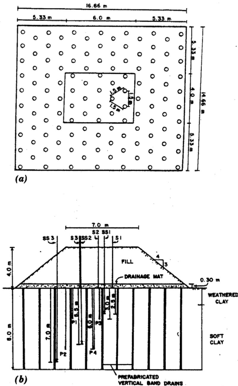
Fig. 14 Embankment plan, section view and layout of field instrumentation at PVD site (Bergado et al. 1992)
