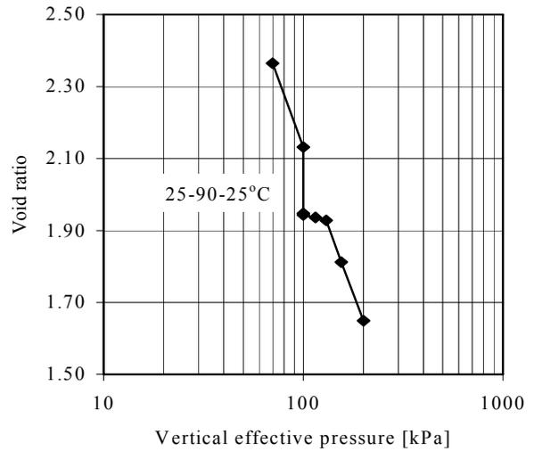
Fig. 2 Temperature induced overconsolidation state of normally consolidated soft Bangkok clay after drained heating/cooling cycle
