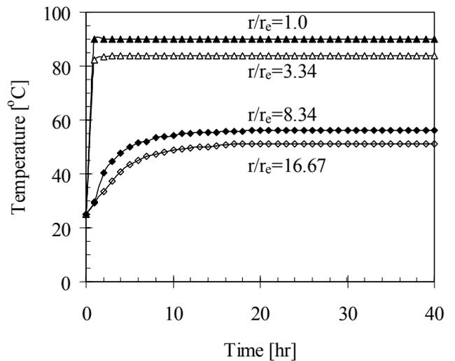
Fig. 10 Temperature change with time at different distances from Thermo-PVD point with constant temperature of 90°C and equivalent radius,  $r_e=6$  mm
