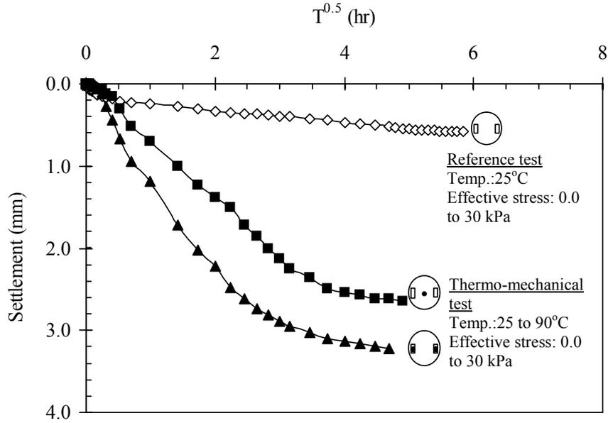
Fig. 13 Thermo-mechanical consolidation test results of reconstituted specimen.
