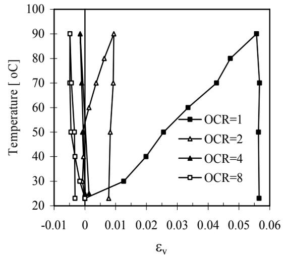
Fig. 1 Soft Bangkok clay temperature volumetric strain under drained heating/cooling cycle at different OCR values (preconsolidation pressure = 200 kPa)
