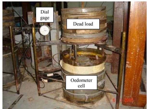
Fig. 5 Large oedometer apparatus
