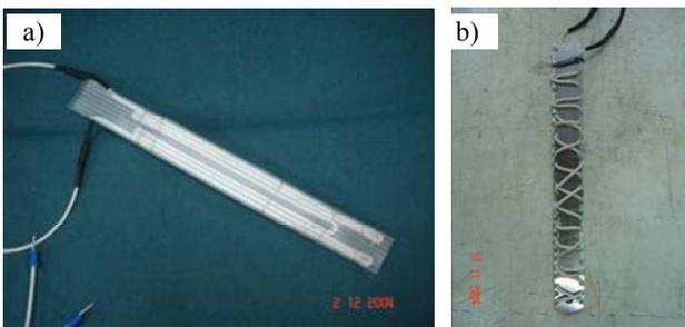
Fig. 7 a) Thermo-PVD configuration; b) Line heat source configuration
