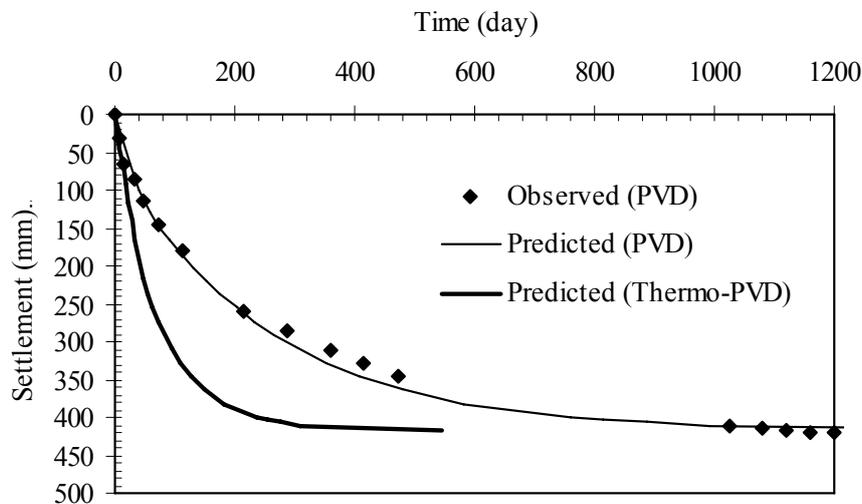
Fig. 15 Comparison between predicted surface settlement using PVD and thermo-PVD system and the observed vertical settlement for PVD system
