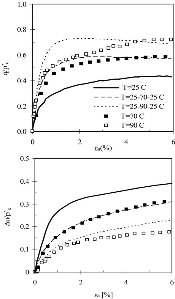
Fig. 4 Undrained triaxial compression test results of normally consolidated soil tested at different temperatures or after subjecting to different heating/cooling cycles
