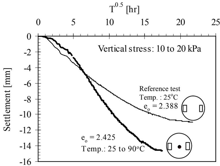
Fig. 12 Thermo-mechanical consolidation test results of reconstituted specimen
