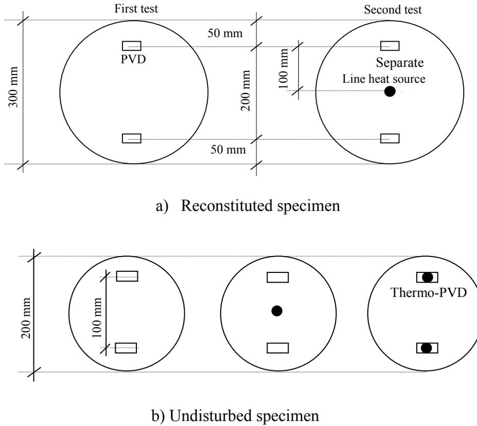
Fig. 8 Thermo-mechanical consolidation test configurations
