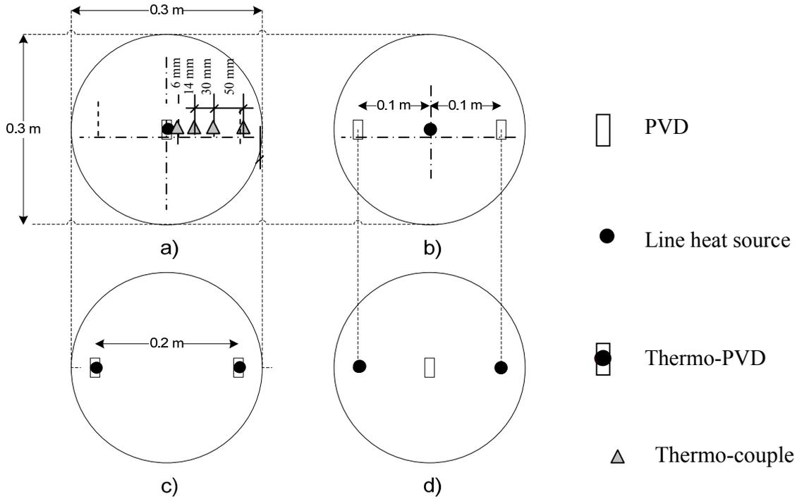
Fig. 6 Different arrangements of Thermo-PVD, PVD, and heater spacing of line heat source in large oedometer cell
