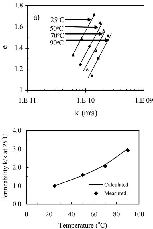
Fig. 3 (a) Effect of temperature on hydraulic conductivity of soft Bangkok clay, (b) effect of temperature on k at constant void ratio
