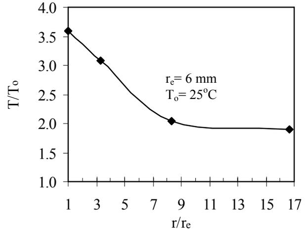
Fig. 9 Temperature-distance relation at steady state condition around thermo-PVD point
