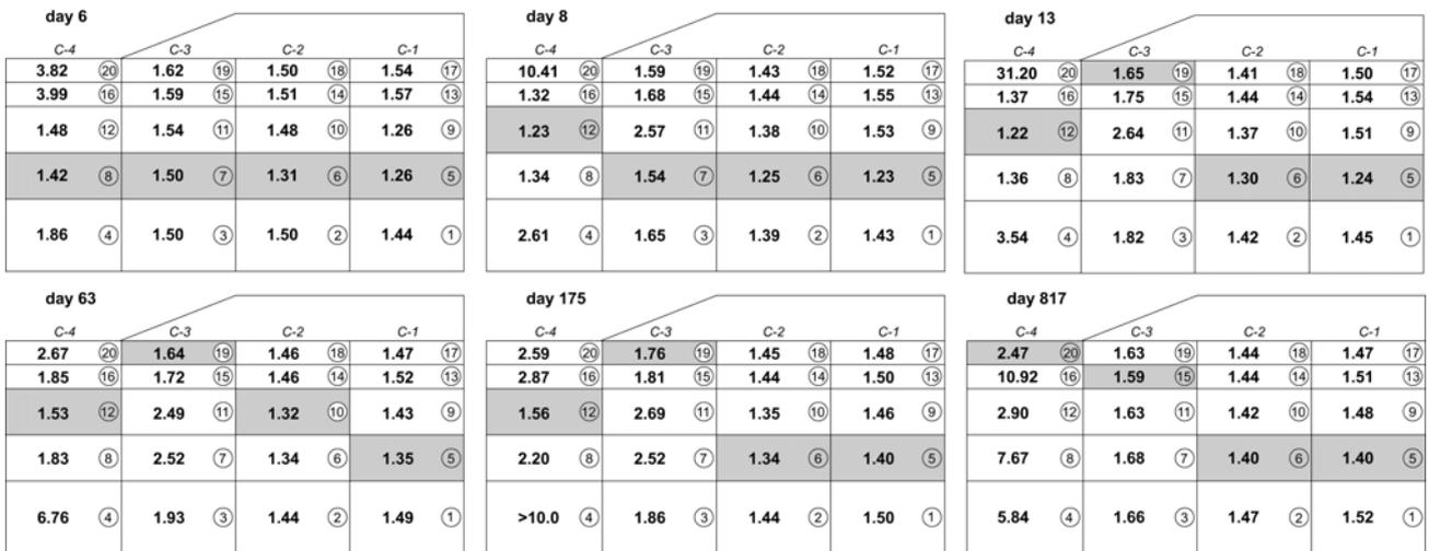
Fig. 8 Safety factors of the soil zones of Cubzac-les-Ponts test embankment B obtained with the Oztoprak & Cinioglu method at different days (shaded zones have the minimum safety factors of the corresponding soil column)
