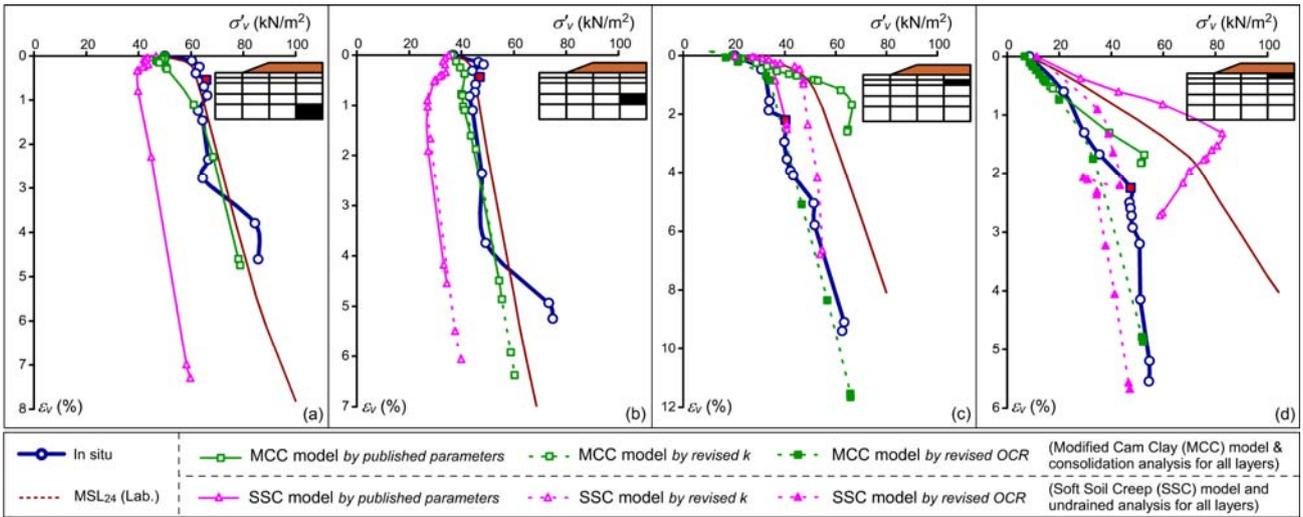
Fig. 4 Comparison of field and laboratory vertical stress – vertical strain relations with those from FE analyses at the foundation soil of Cubzac-les-Ponts Embankment
