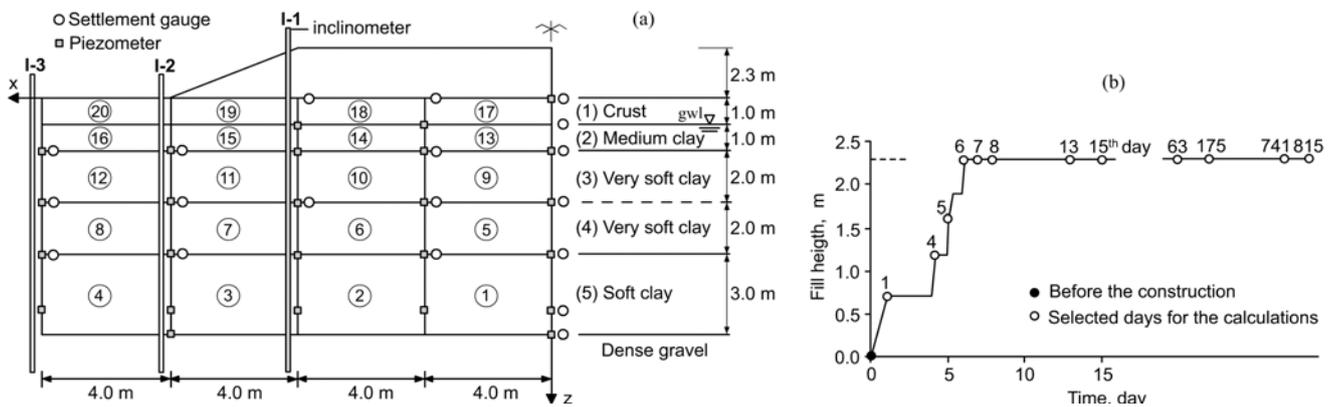
Fig. 2 Cubzac-les-Ponts embankment (a) Zonation system according to the soils and instrumentation, (b) Construction history
