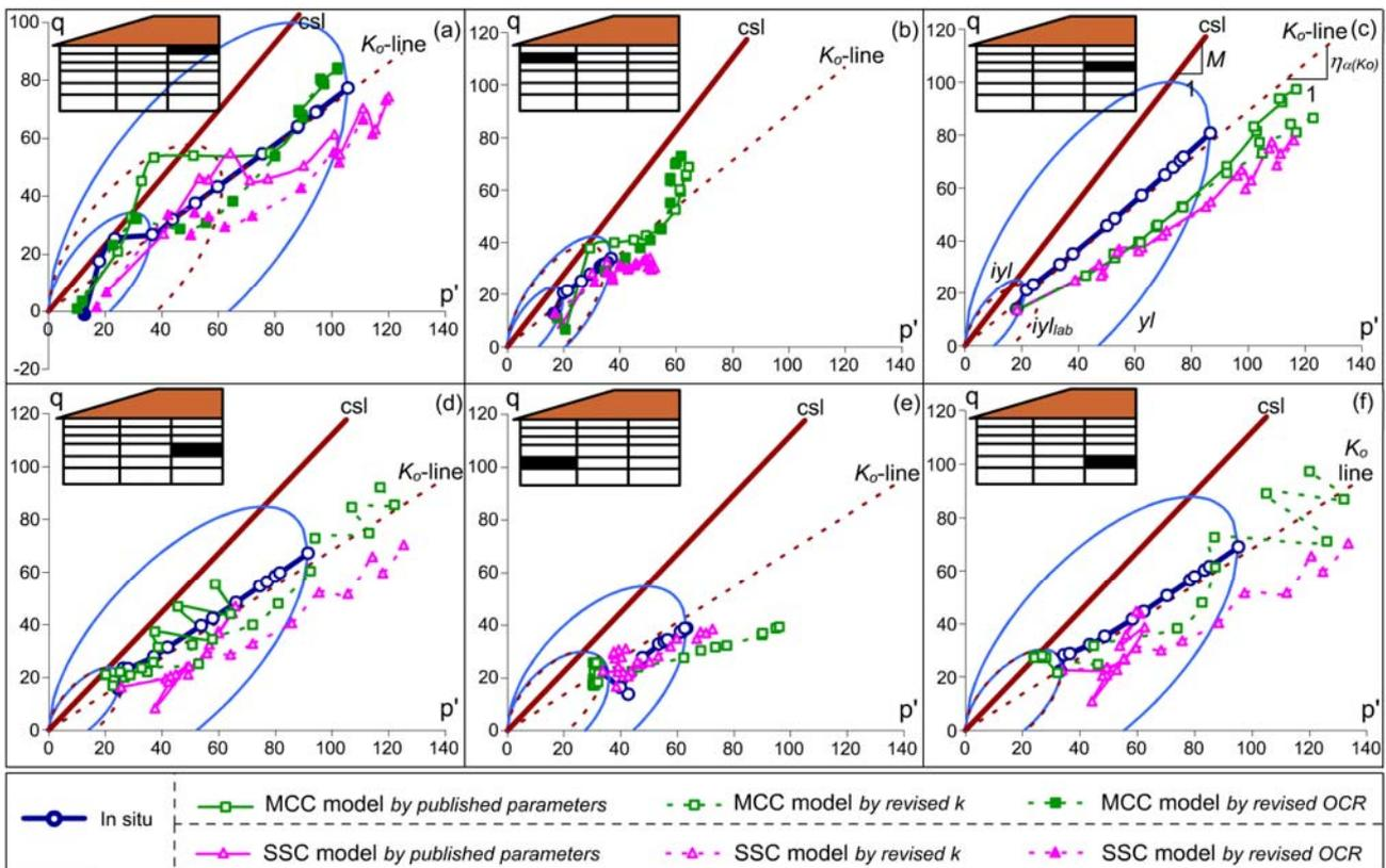
Fig. 7 Achieved stress paths by the Oztoprak & Cincicioglu method and calculated ones with FE analysis on the  $q-p'$  plane for various zones in the foundation soils of Stanstead Abbots embankment ( $iyl$ ,  $iyl_{lab}$ ,  $yl$ ,  $csf$ , and  $K_0$ -line are located by the Oztoprak & Cincicioglu method;  $iyl$ : initial in situ yield locus,  $iyl_{lab}$ : initial yield locus obtained from  $MSL_{24}$  test,  $yl$ : outer in situ yield locus)
