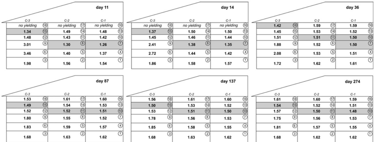
Fig. 9 Safety factors of the soil zones of Stanstead Abbots Embankment obtained with the Oztoprak & Cinioglu method at different days (shaded zones have the minimum safety factors of the corresponding soil column)
