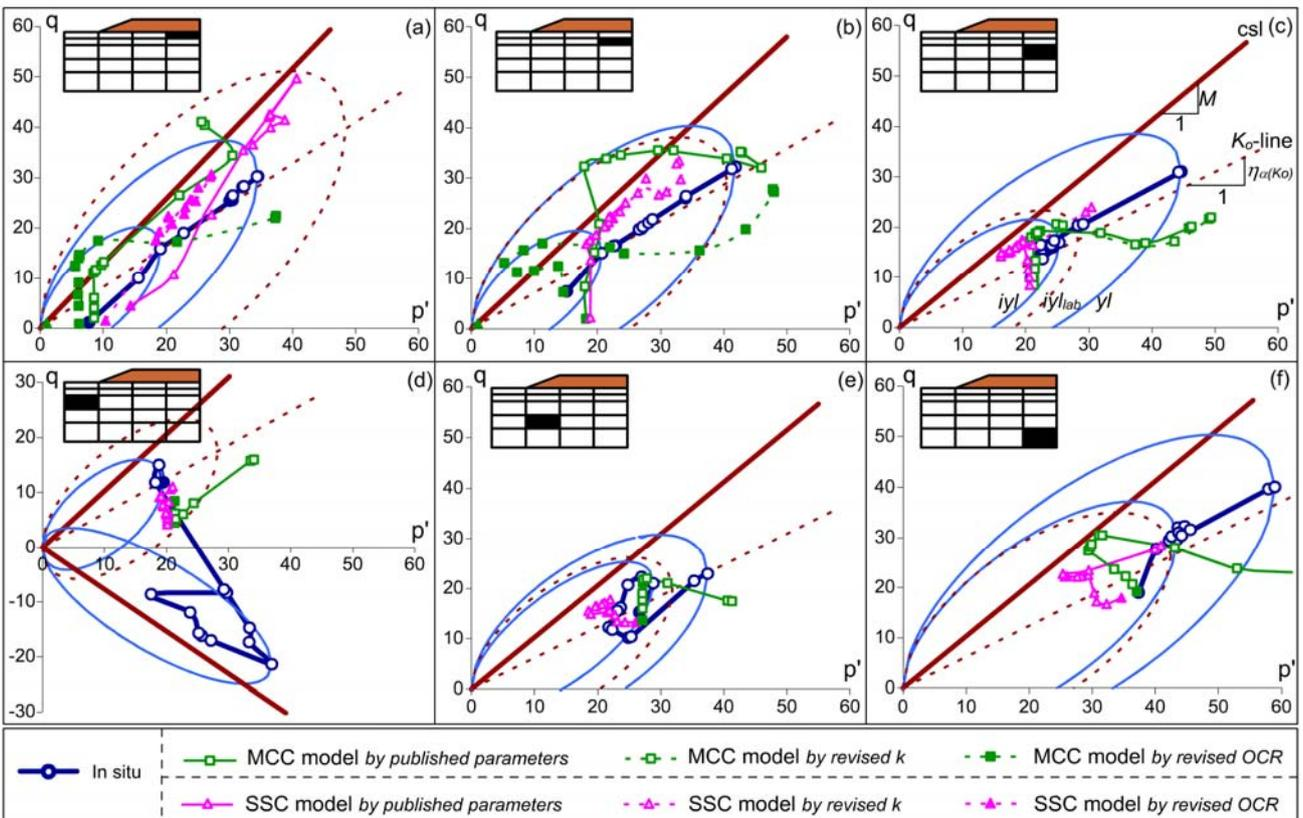
Fig. 5 Achieved stress paths by the Oztoprak & Cinicioglu method and calculated ones with FE analysis on the  $q-p'$  plane for various zones in the foundation soils of Cubzac-les-Ponts test embankment B ( $iyl$ ,  $iyl_{lab}$ ,  $yl$ ,  $csl$ , and  $K_{\sigma_z}$ -line are located by the Oztoprak & Cinicioglu method;  $iyl$ : initial in situ yield locus,  $iyl_{lab}$ : initial yield locus obtained from  $MSL_{24}$  test,  $yl$ : outer in situ yield locus)
