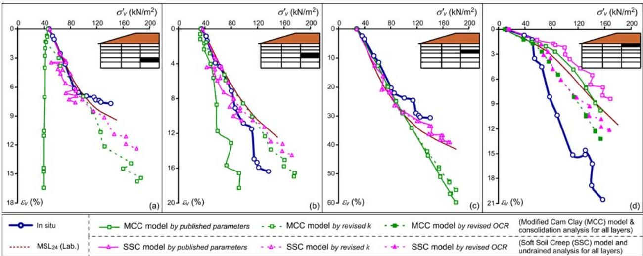
Fig. 6 Comparison of in situ and laboratory vertical stress – vertical strain relations with those FE analyses at the foundation soil of Stanstead Abbots embankment
