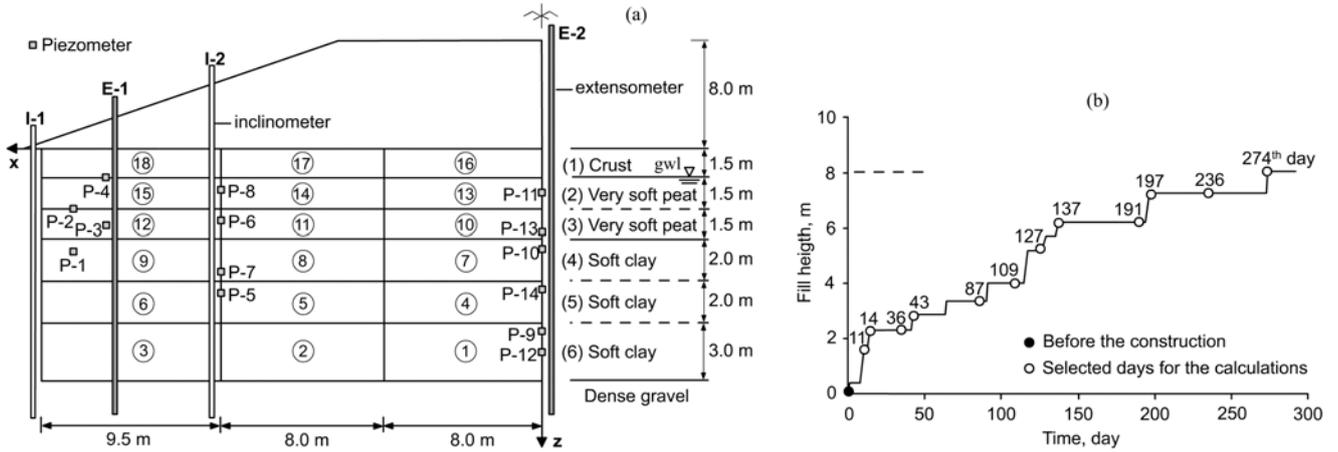
Fig. 3 Stanstead Abbots embankment (a) Zonation system according to the soil properties and instrumentation, (b) Construction history
