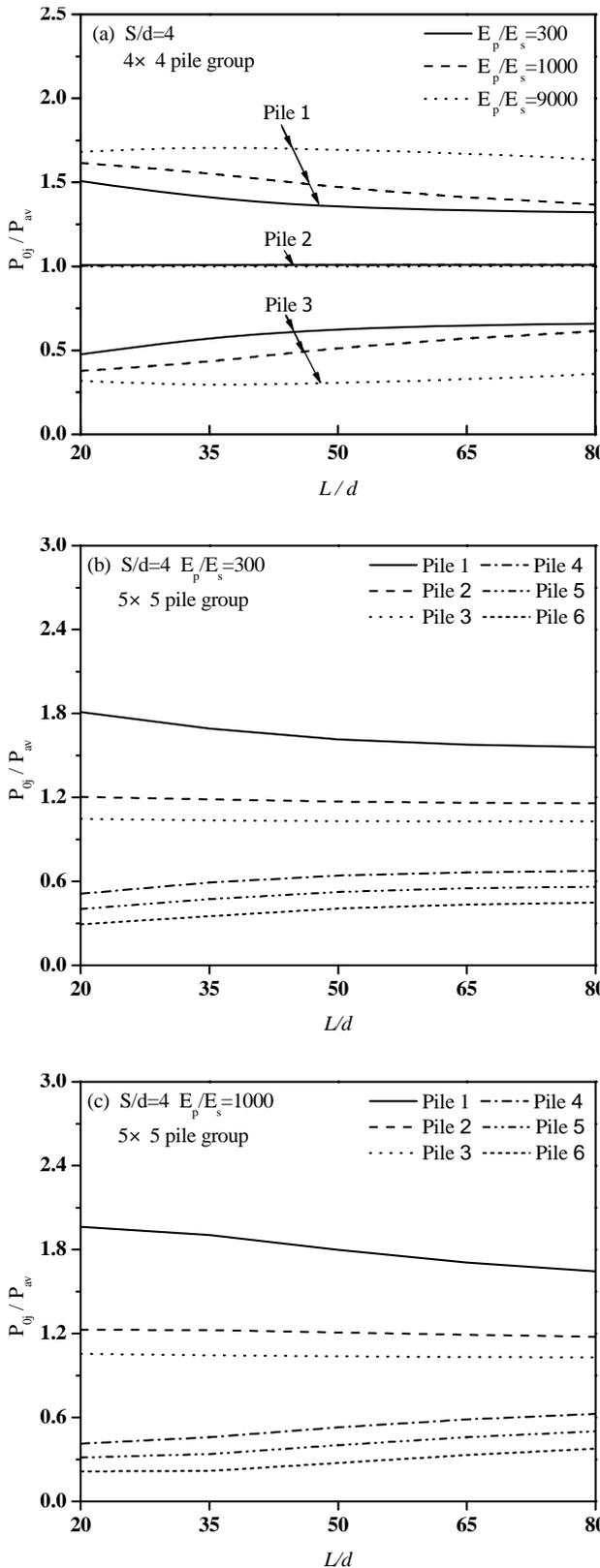
Fig. 7a Load distribution versus pile slenderness ratio
