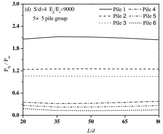
Fig. 7b Load distribution versus pile slenderness ratio
