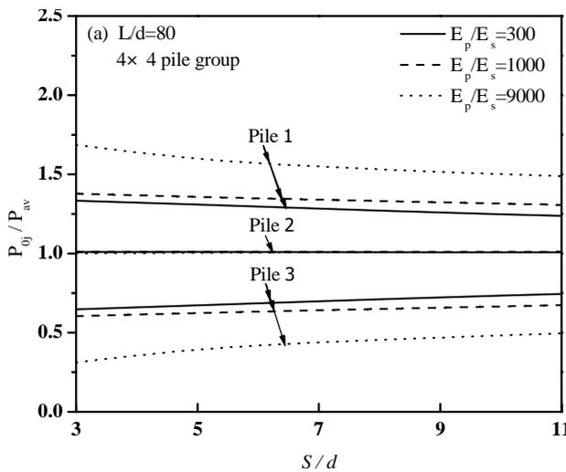
Fig. 6a Load distribution versus pile spacing ratio
