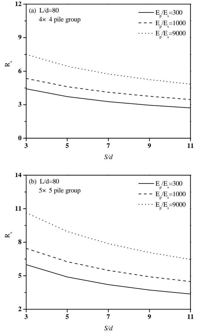
Fig. 4 Pile group settlement ratio versus pile spacing ratio
