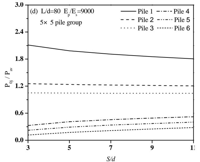
Fig. 6b Load distribution versus pile spacing ratio
