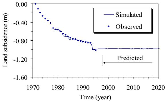
Fig. 11 Predicted land subsidence when pumping with the optimal yield
