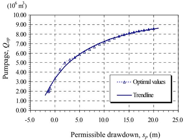
Fig. 10 Optimal pumping under varying drawdown
