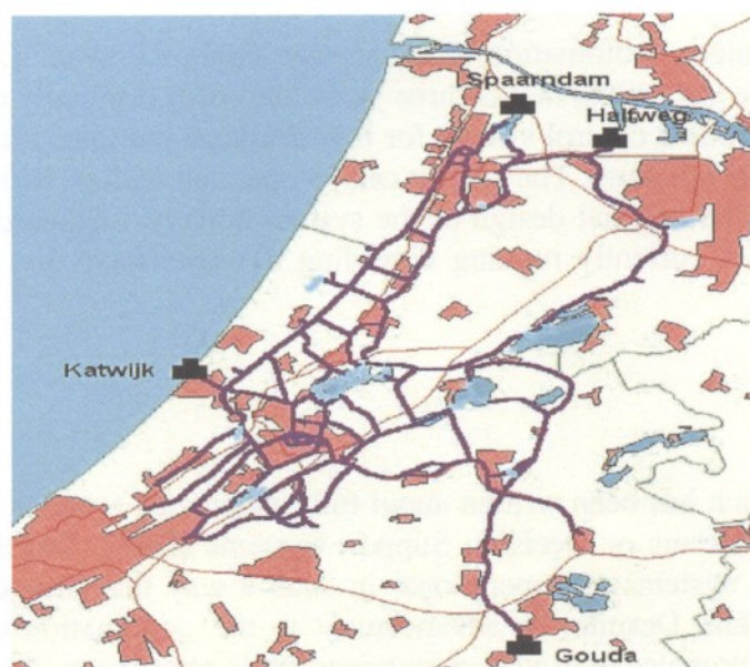
Fig. 1 The canal network of Rijnland, called bossom canals, is controlled by four drainage pumping stations (capacity 150 m 3 /s). The aim of the project was to build a Real Time Control system for the operation of the pumping stations.
