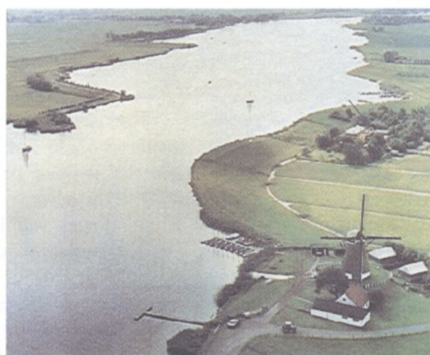
Fig. 4 Impression of an older part of the bossom canal in Rijnland. The allowable water level fluctuation in the basin is only 0.05 m.
