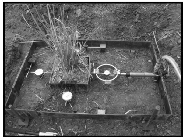
Fig. 4 Field direct shear test equipment
