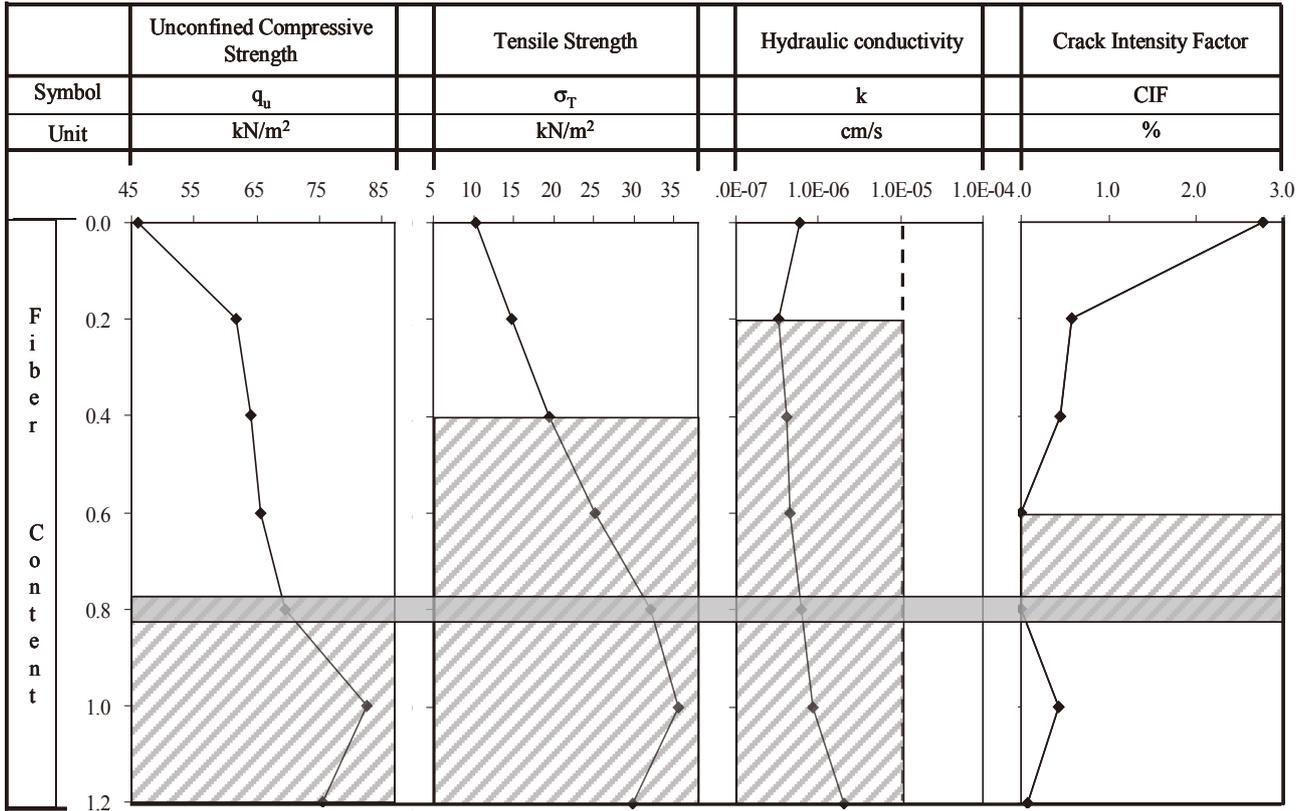
Fig. 8 Overall acceptable zones for the compacted soil-fiber mixtures
