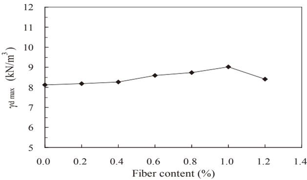
Fig. 3 Change in  $\gamma_{d max}$  with various fiber
