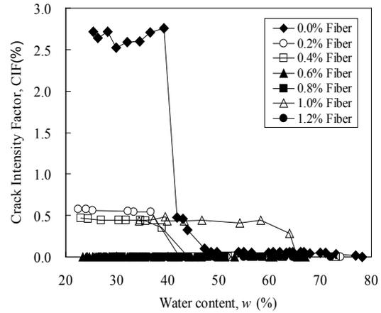
Fig. 7 Crack intensity factor for various fiber contents
