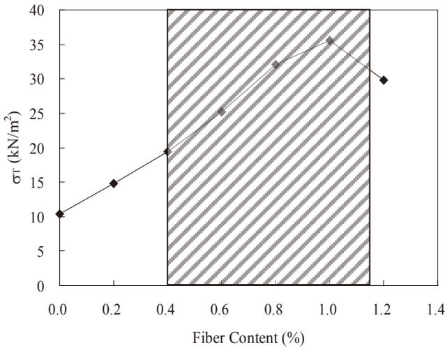
Fig. 5 Acceptable zone based on tensile strength consideration
