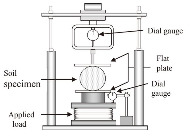
Fig. 1 Schematic of the modified indirect tensile apparatus
