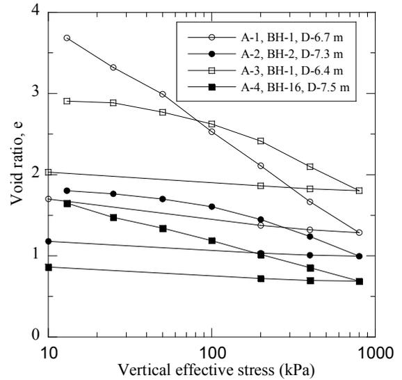
Fig. 4 Typical e-logP curves of organic clay samples
