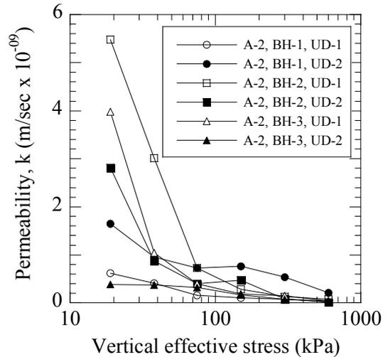
Fig. 7 Coefficient of permeability ( $k$ ) vs. vertical effective stress
