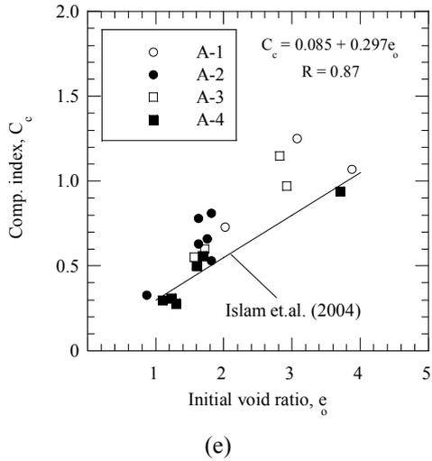
Fig. 8 (a) Correlations of unconfined compressive strength ( $q_u$ ) with SPT N-value; (b) correlations of unconfined compressive strength ( $q_u$ ) with plasticity index (PI); (c) correlations of unconfined compressive strength ( $q_u$ ) with organic content; (d) correlation of compression index ( $C_c$ ) with organic content and (e) correlation of compression index ( $C_c$ ) with initial void ratio ( $e_0$ )
