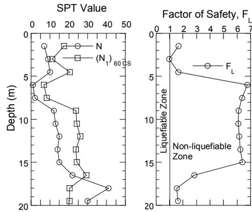
Fig. 9 Liquefaction potential evaluated based on SPT
