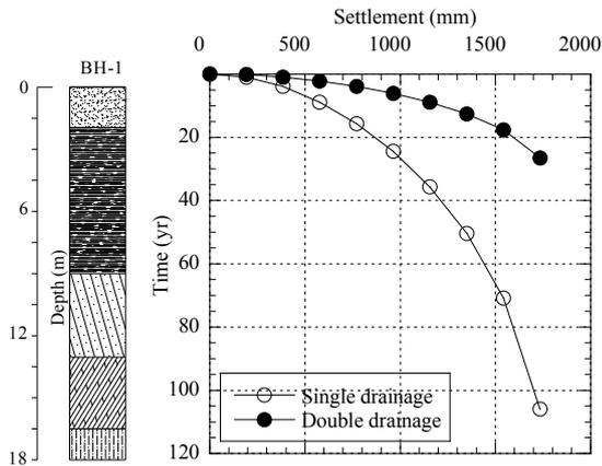
Fig. 10 Typical curves of time dependant settlement of soft organic layer due to the surcharge from filling layer (A-1/BH-1).
