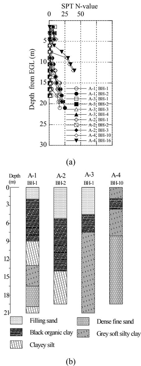
Fig. 2 (a) Variation of SPT N-value with depth from EGL and (b) typical borelogs of different study areas
