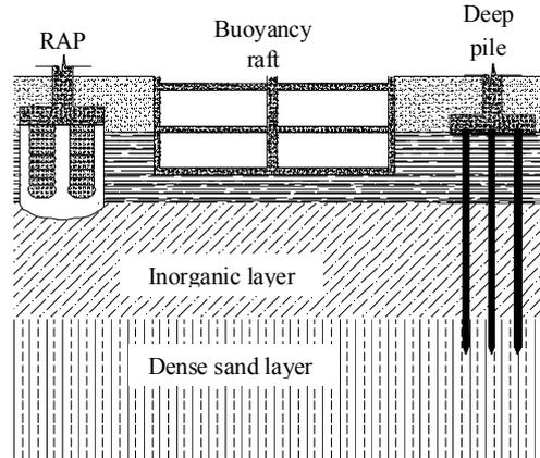
Fig. 11 Suitable foundation systems for the study area
