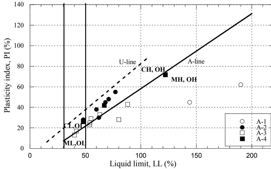
Fig. 3 Position of the cohesive soil samples on Casagrande plasticity chart
