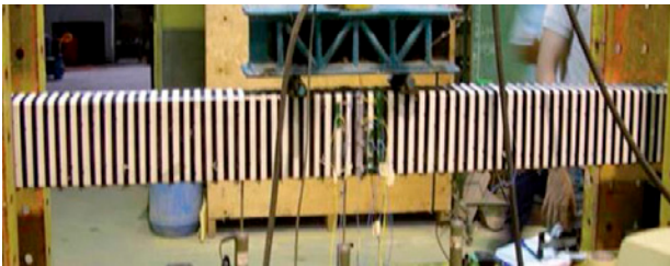
Fig. 8. Strengthening of over-reinforced HSC RC beam using PTMS to prevent concrete crushing failure (after Ma et al., 2015).
