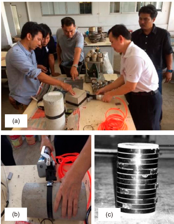
Fig. 12. (a)-(b) Post-tensioning strapping, and (c) view of PTMS-confined cylinder.
