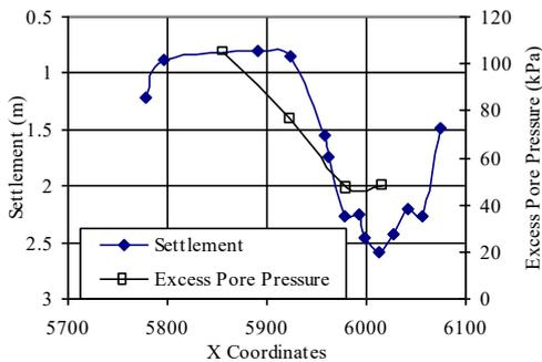
Fig. 6. Boundary Effects Measured by Settlement Plates and Piezometers installed across The Pilot Area.
