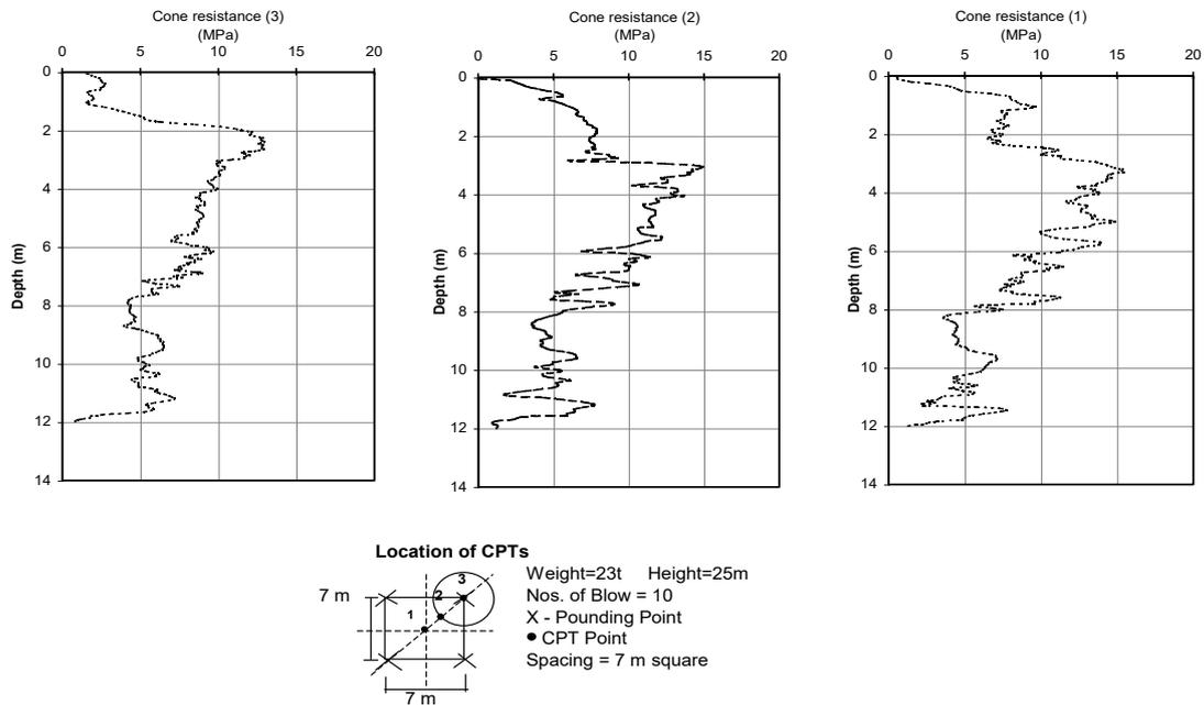
**Fig. 11.** Cone resistance results after dynamic compaction (after Choa et al. 2001).
