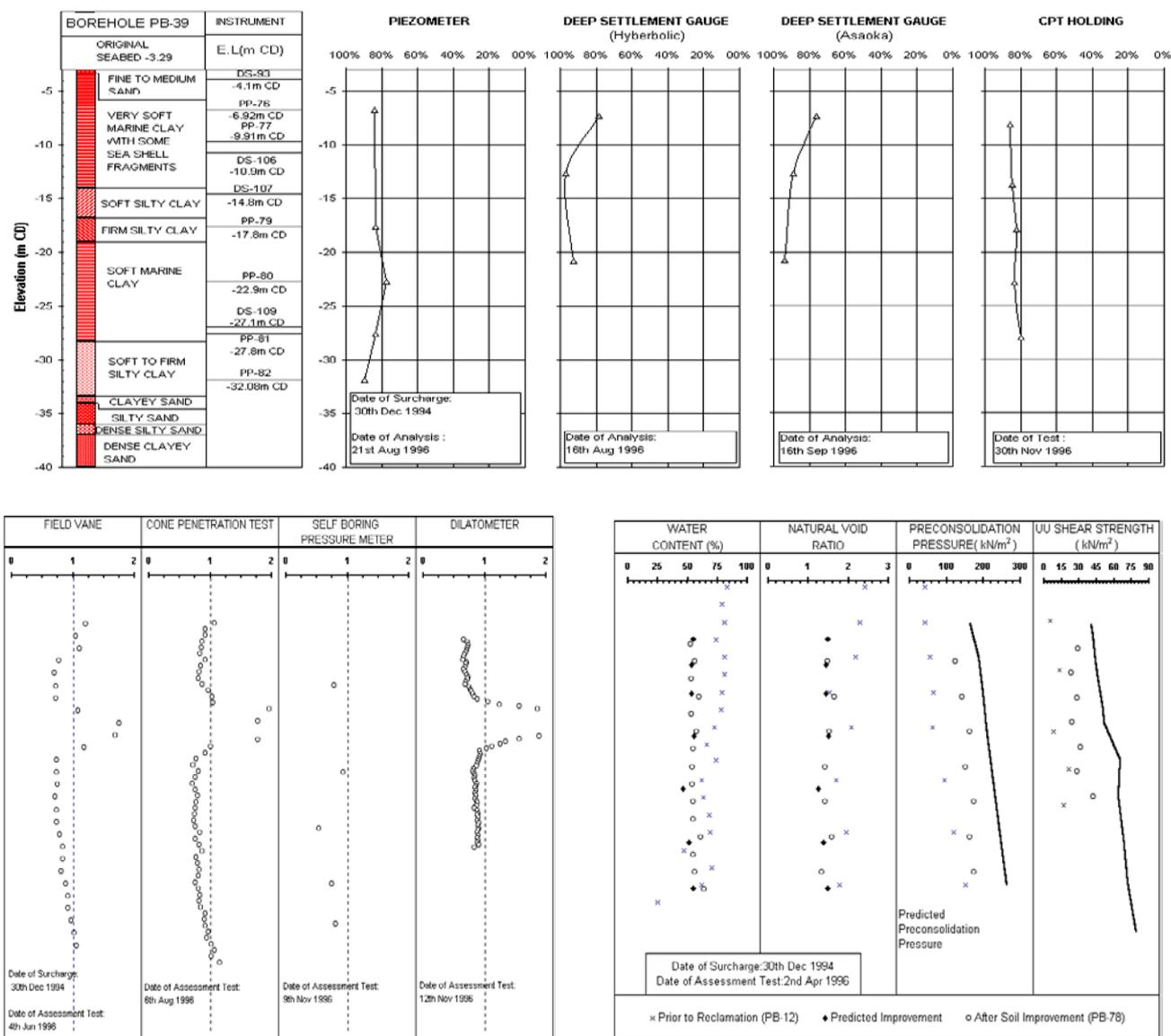
**Fig. 9.** Assessment of Ground Improvement Using Geotechnical Instrument and Filed Investigation Data.
