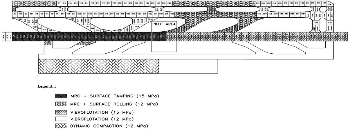
**Fig. 10.** Areas Showing Deep Compaction Carried Out by 3 Different Compaction Methods.
