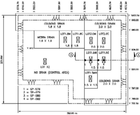
Fig. 3. Layout of Third Pilot Area in Phase 1C.
