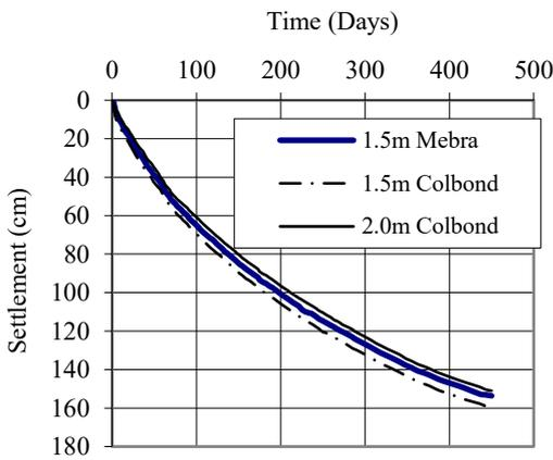
Fig. 4. Same magnitude and rate of settlement caused by various types of drain under same boundary condition.
