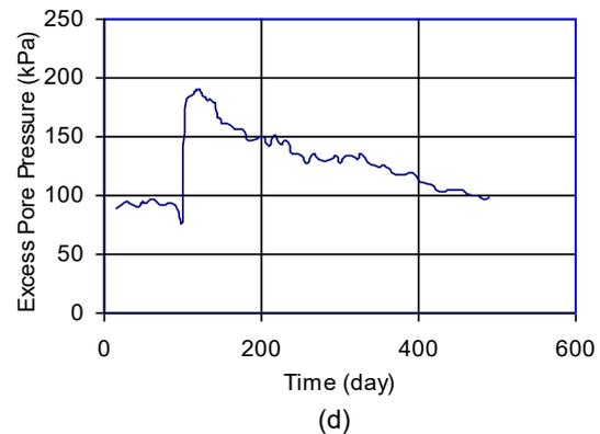
Fig. 7. Pilot Area (Area A North) Using Dredged Clay Fills (a) Profile of Fill (b) Filling Sequence (c) Settlement Vs time (d) Pore Pressure Vs Time.
