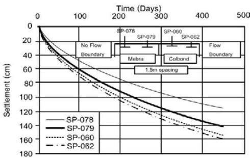
Fig. 5. Different magnitude and rate of settlement caused by different boundary condition.
