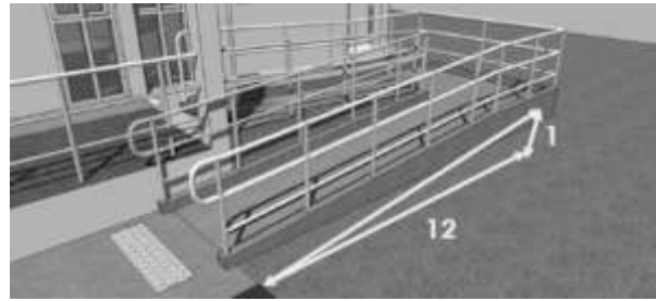
Fig. 3. General ramp with 1:12 slope.
