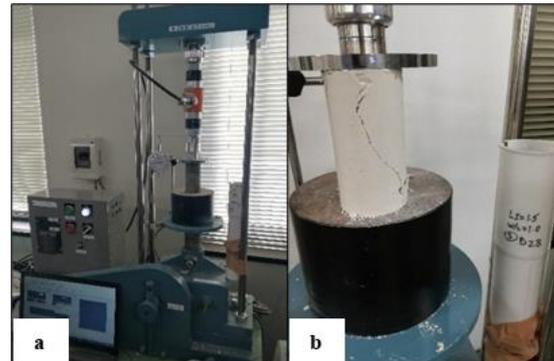
Fig.5: Load & displacement measurement device
