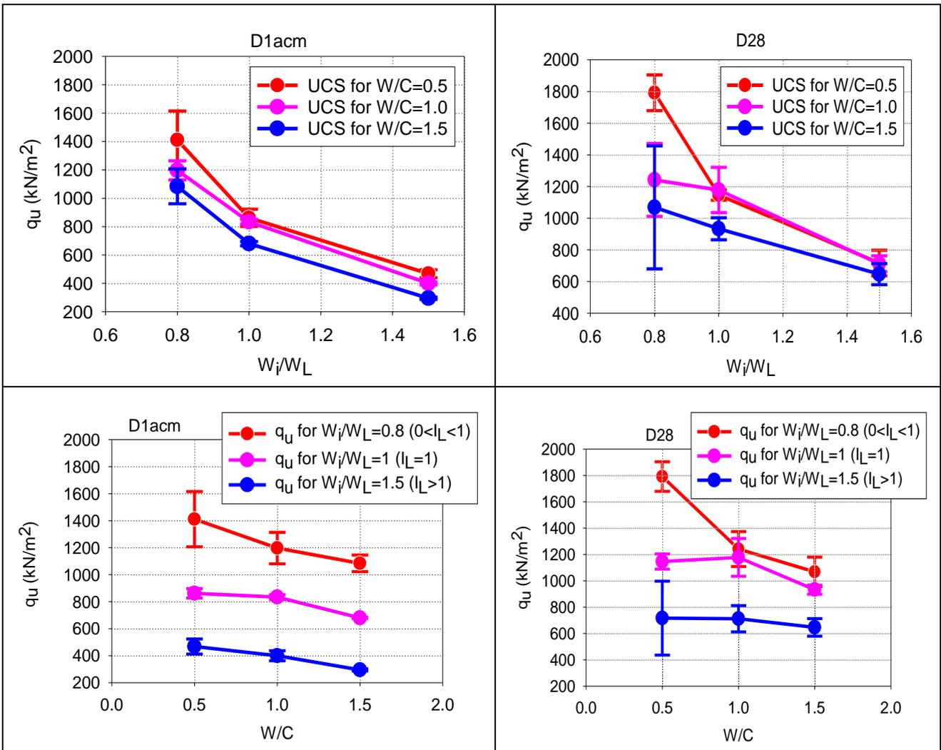
Fig.8: UCS with standard deviation error bars in function of  $W_i/W_L$  and  $W/C$  for D1acm and D28.
