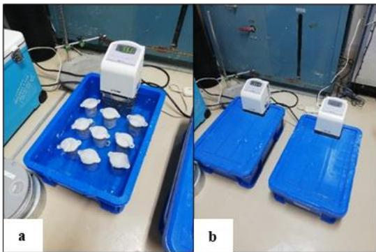
Fig.4: Constant temperature water tanks
