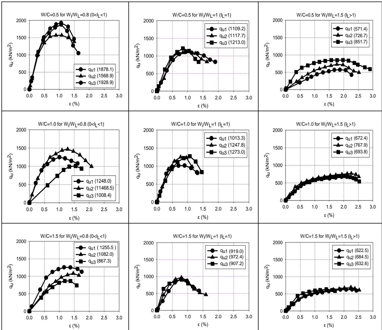
Fig.6: UCS of D28 for each  $W_f/W_L$  and each W/C in function of strain  $\epsilon$ .
