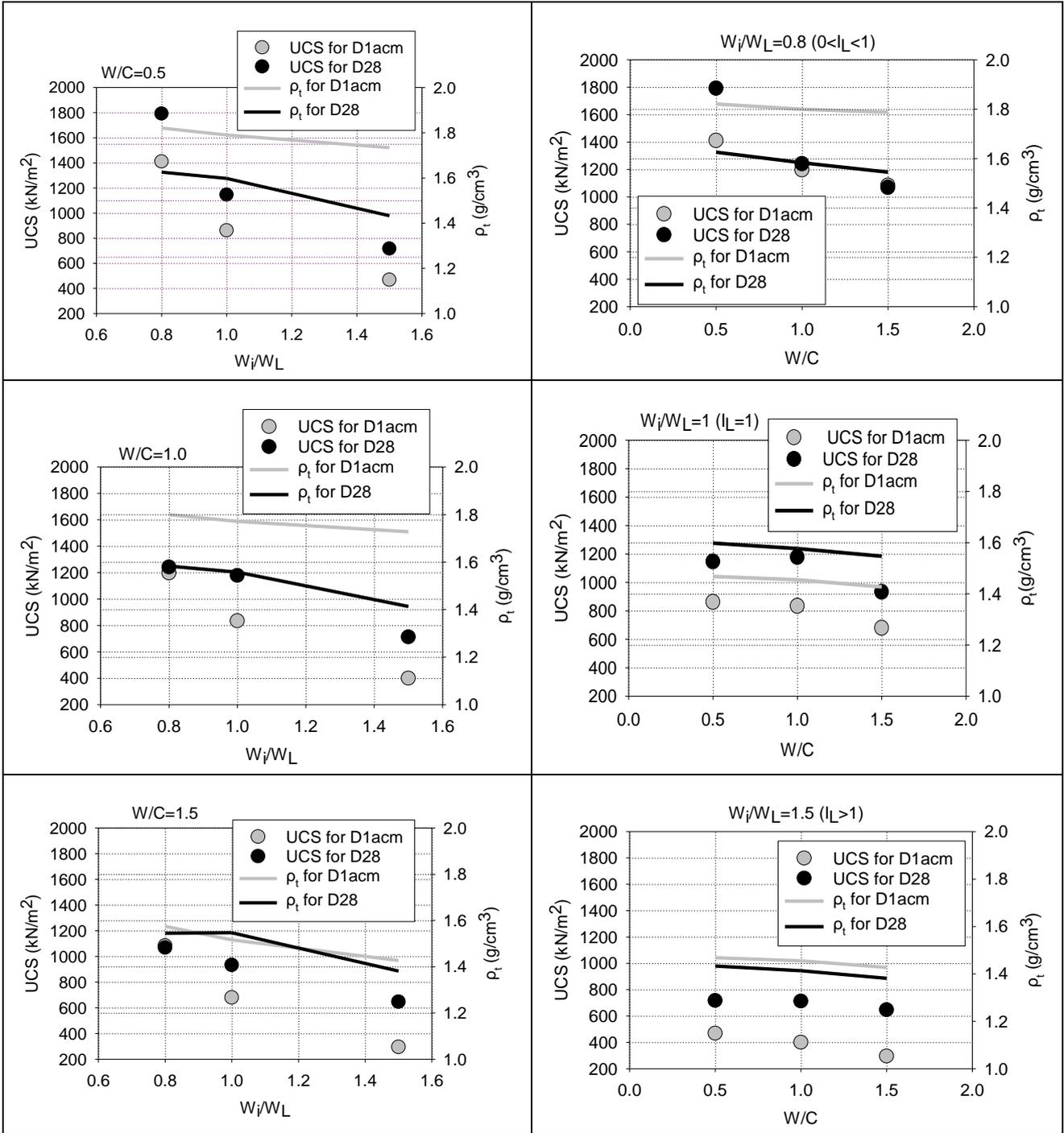
Fig.7: UCS and wet density  $\rho_t$  for each  $W_i/W_L$  and each  $W/C$  about D1acm and D28.
