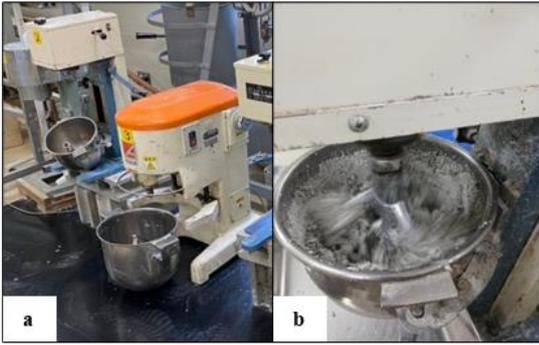
Fig.2: Electrically operated mixer
