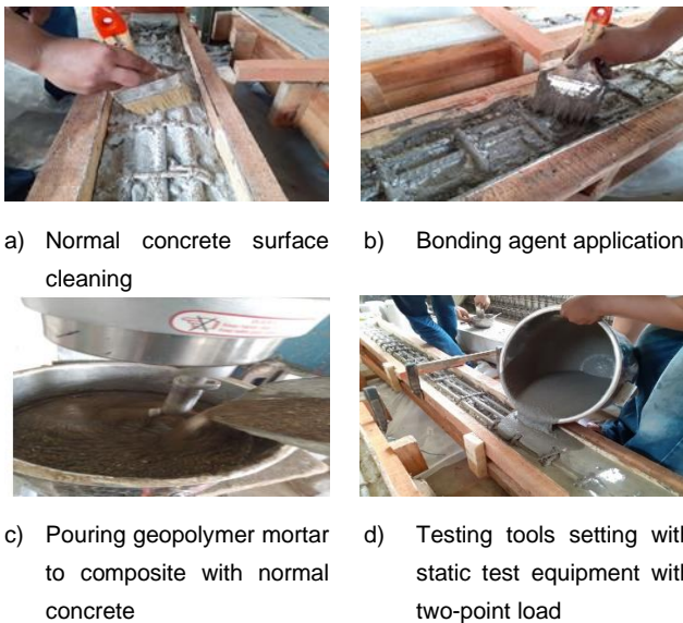
Figure 2. Geopolymer mortar mixing process
