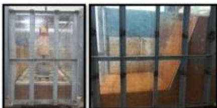
Fig. 1. Soil Compaction and Slope Construction
