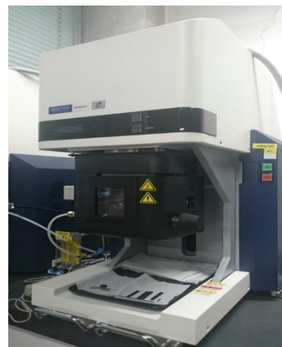
Figure 2. Experimental equipment used in vibration test (DMA7100, HITACHI)
