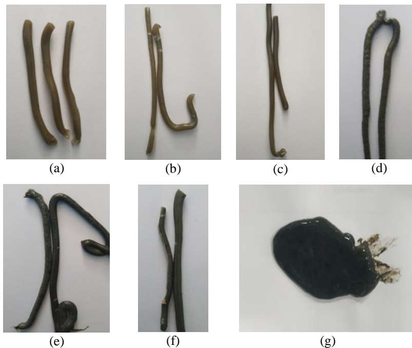
Figure 4. Result of melting by different temperature (a) 170°C (b) 180°C (c) 190°C (d) 200°C (e) 210°C (f) 220°C (g) 230°C
