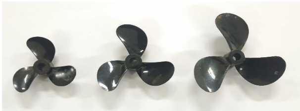
Figure 5. Propeller models FPP; Diameter a). 32 mm, b). 40 mm, c). 48 mm
