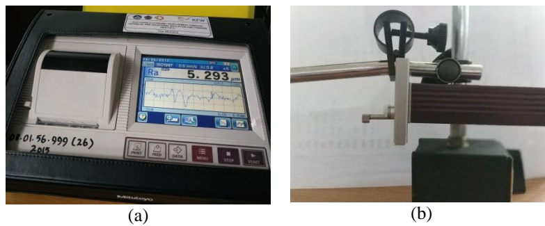
Figure 5. (a) Portable surface roughness testing machine SJ-310 Mitutoyo (b) detector of surface roughness attached by dial indicator base
