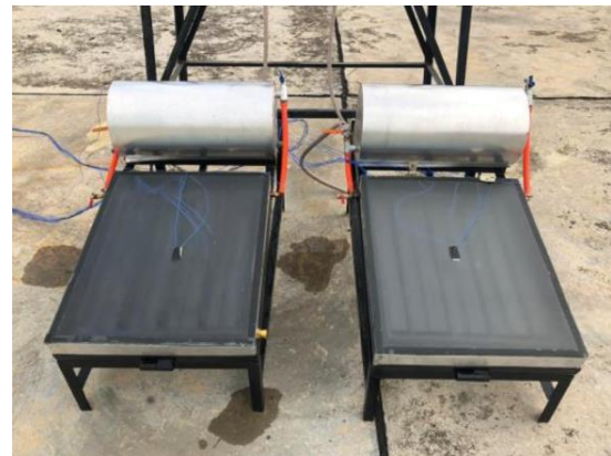
Figure 8. Absorber plate with PCM storage (left side) and without PCM storage (right side)
