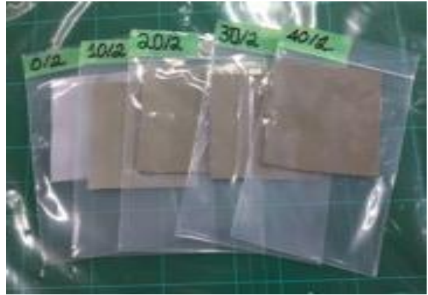
Figure 3. Sample of silicon rubber with coal fly ash filler
