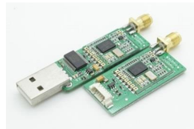
Figure 4. Radio Telemetry 433 Mhz
