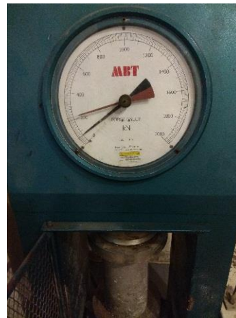
Figure 6. Compressive strength test
