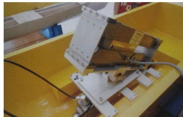
Figure 2. The resistance dynamometer R35E as attached on model
