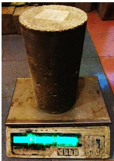
Figure 5. Concrete weight measurement
